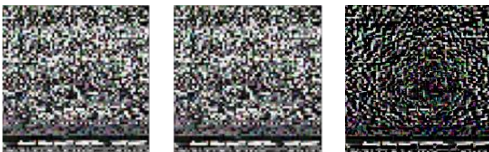
FIGURE 9: Yuner.A original (left) and the generated adversarial attack image (center) – virtually indistinguishable; and the difference between the two highlighted (right).
