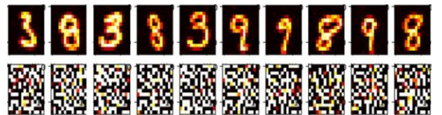
FIGURE 4: Top row: original samples of handwritten characters. Bottom row: reconstructed using non-random back-projection from second layer (64-dimensional feature).
