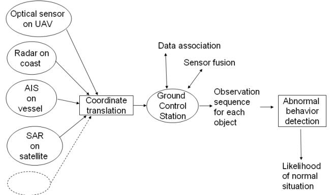
Figure 3. The sensors perform data processing, detection, tracking and feature classification. The Ground Control Station (GCS) performs track association, track fusion, attribute fusion and abnormal behaviour detection.
