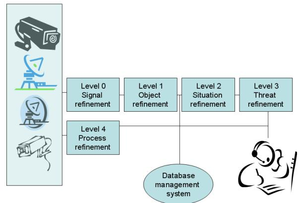
Figure 1. Structure of the JDL model.
