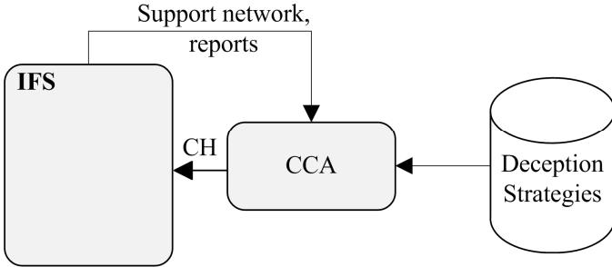
Fig. 5. Outline of the interfaces of a CCA that could produce the CH of (6) . It receives the support network and intelligence reports from the IFS. An archive of deception strategies is available.
