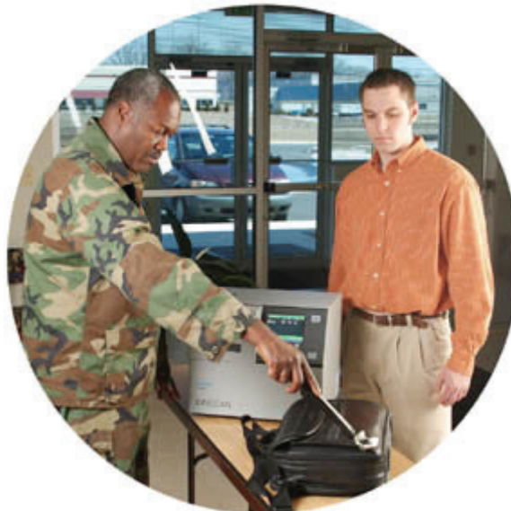
Figure 1: Swiping a bag for particles for detection with Smiths Detection IonScan 400B (Courtesy of Smiths Detection)
