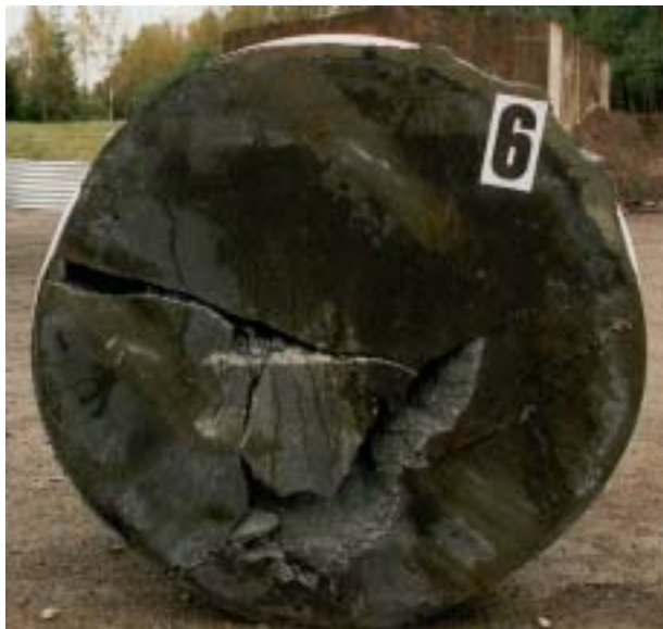
Figure 33. Post condition for back face of target 3 (shot 6).
