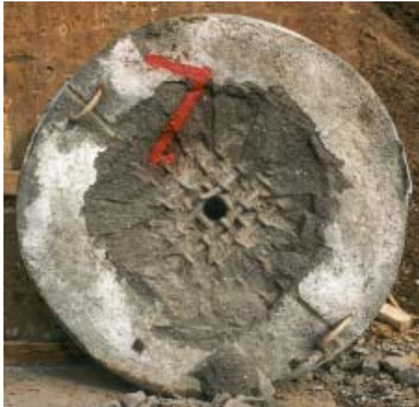
Figure 56. Post condition for front face of target 7 (shot 7).
