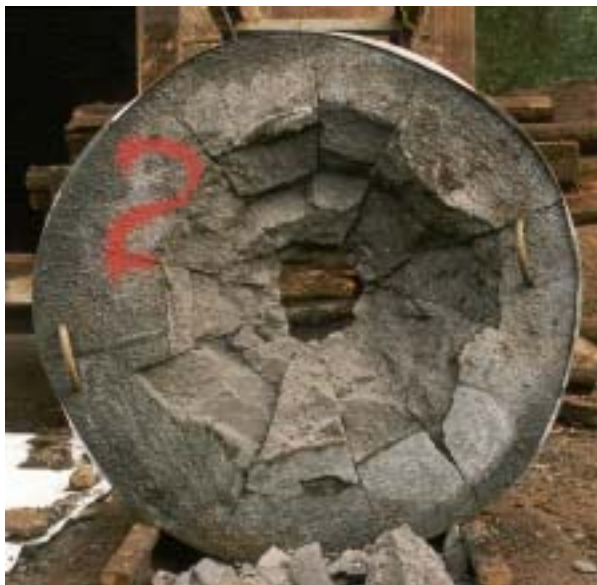
Figure 44. Post condition for front face of target 5 (shot 2).
