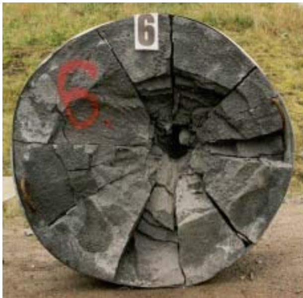
Figure 31. Post condition for front face of target 3 (shot 6).
