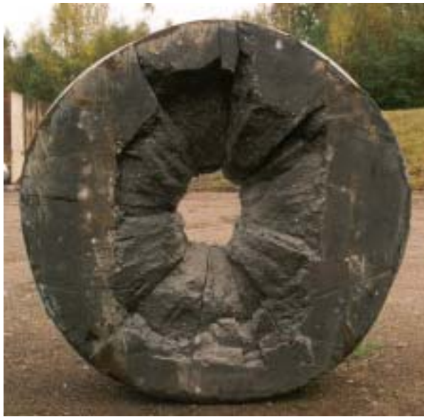
Figure 46. Post condition for back face of target 5 (shot 2).
