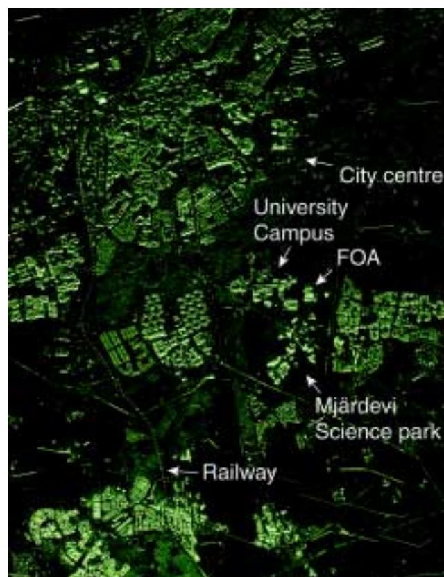
Figure 18. Image over Linköping processed with the factorized back-projection algorithm.
