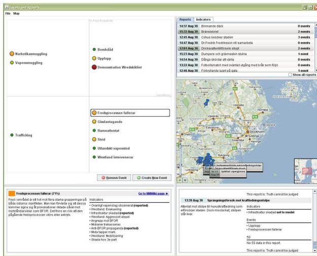
Fig. 3. This picture shows the Impactorium GUI. Monitored events are shown top left, sorted according to their estimated severity and a priori probability. Bottom left, more details on a selected event are shown. On the right, a list of reports, report positions on the map, and details of selected report are shown. It is also possible to select the indicator tab (top right) and see details on the currently active indicators instead of reports.
