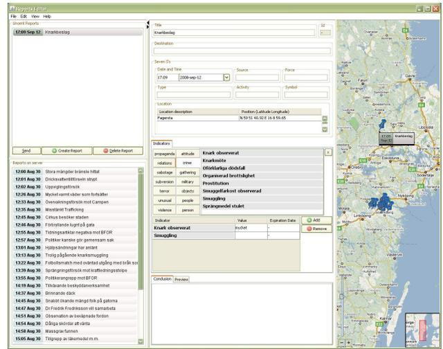
Fig. 2. The GUI of the Reportorium tool. A list of reports is shown on the left, while the middle pane is used to edit new reports. The map to the right allows the user to associate the report with a geographical position.
