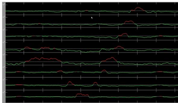
Figure 2. PAT detector output, from the eight hydrophones in the tripwire (time on the x-axis). The results are from a trial in the port of Gothenburg in May 2013. Graphs are red when detector output is above the threshold.
