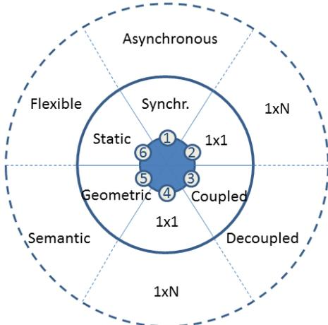
Figure 1. The inner circle represents the typical parameter values of DA (i.e., the DA values for target tracking). The outer circle (with its dashed boundary) illustrate how these parameters are relaxed for gDA.
