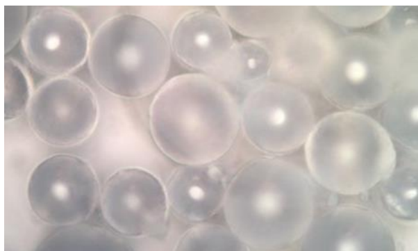
Figure 3. Improved 100% dense ADN prills with reduced sensitivity.
