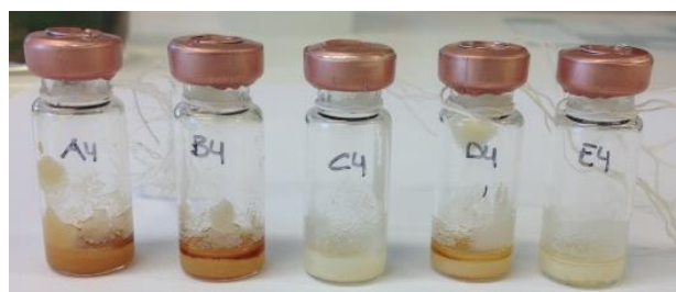
Figure 5. ADN/polymer compatibility testing after 21 days at 75°C.
