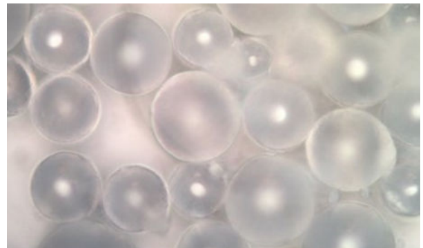
Figure 13. Improved 100% dense ADN prills with reduced sensitivity.
