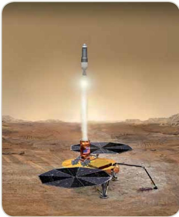
Solid propellant is considered for the Mars ascend vehicle.
