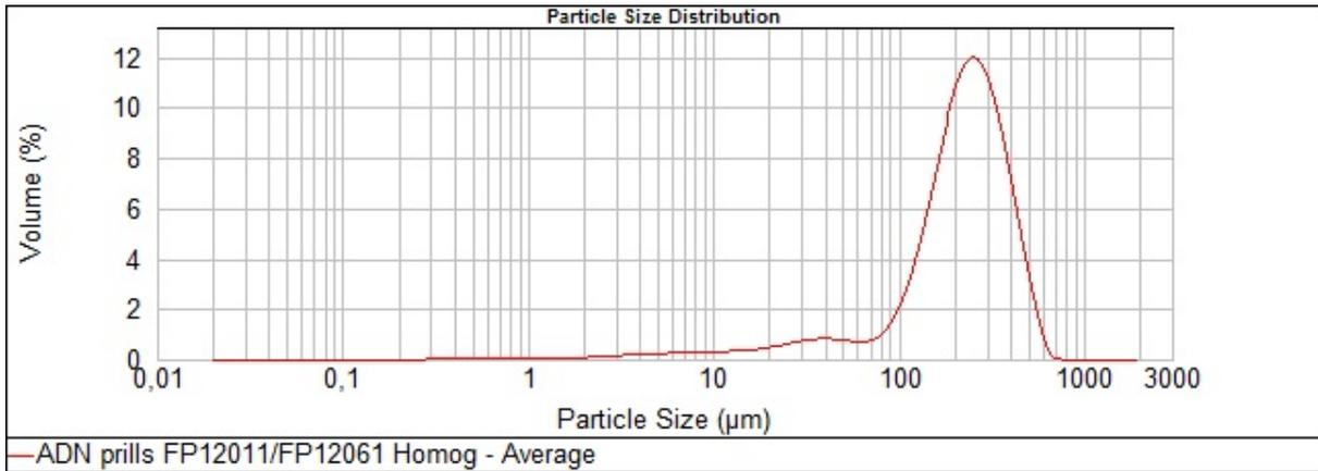
**Figure 1.** Result from particle size distribution measurement.
