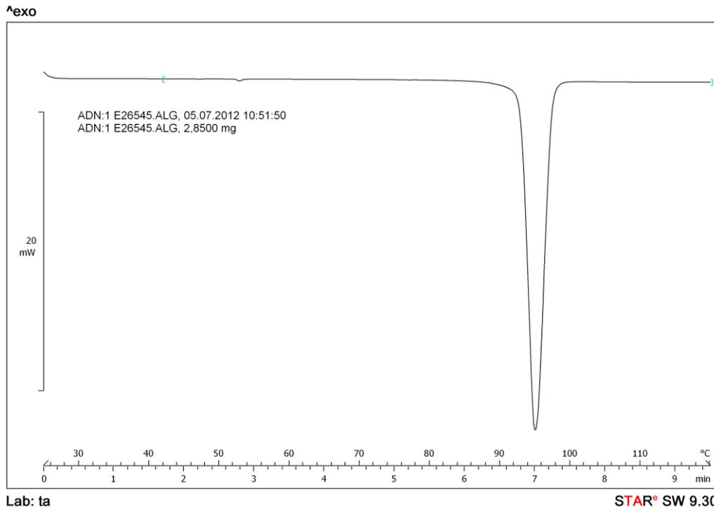
**Figure 2.** DSC thermogram for prilled ADN, batch FP12011/FP12061, at a heating rate of 10 K/min.
