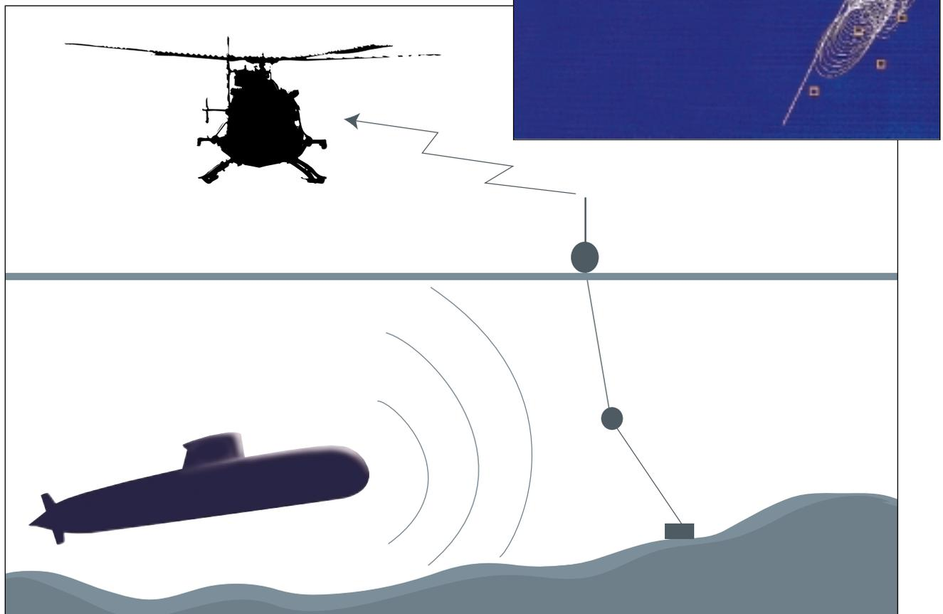
**Fig 4 and 5.** Passive, non-directional sonobuoys are launched into the sea from a helicopter which tries to track a submarine in the shallow and acoustically very complex waters of an archipelago. The sonobuoys have to be dropped at locations quite close to the submarine (probably as close as 100-300 meters).
