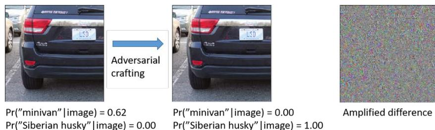
**Figure 1: From minivan to Siberian husky. The absolute difference (amplified a factor 20) between the original and manipulated (adversarially crafted) image is shown to the right. The adversarial example (center) is generated using Kurakin’s basic iterative method (BIM) described in [28].**
