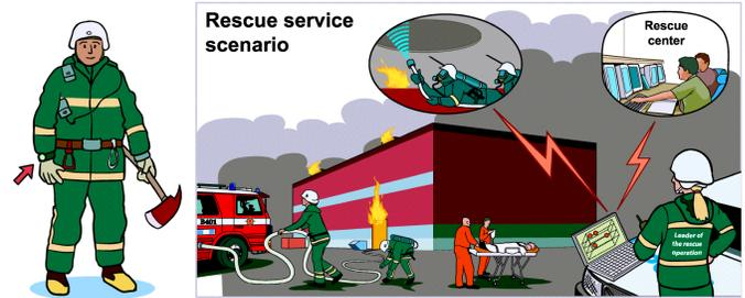
Fig. 3. In this scenario on-body sensors are primarily monitoring the vital status of fire fighters and rescue personnel in dangerous environments. Sensors can also be used to monitor the location of the individual fire fighters as well as external environment, e.g. ambient temperature, oxygen content, chemical 'sniffers' for explosive gases, etc.
