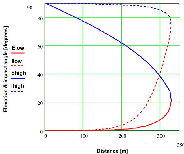
**Figure 5. Elevation (solid line) and impact angle (dashed line) as function of distance. Low trajectories are red and high trajectories blue.**
