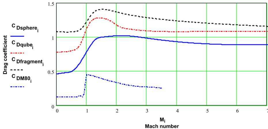
Figure 6. Aerodynamic drag coefficient for three different fragment types and M80 7.62 mm bullet.
