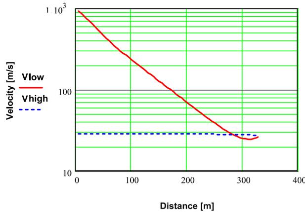
**Figure 4. Velocity as a function of impact distance. The low trajectory is solid red and the high trajectory dashed blue.**
