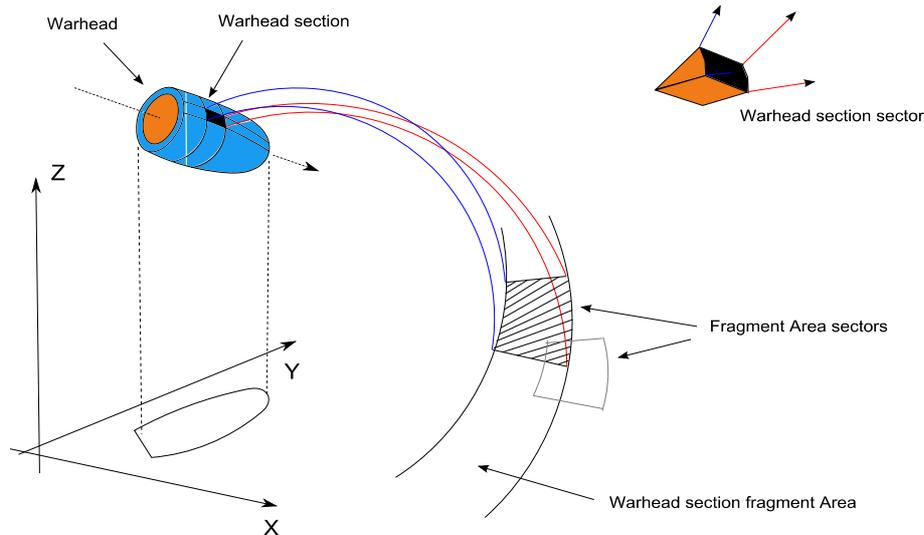
Figure 3. Calculation of fragment density, here illustrated for one radial sector, from a single warhead section, and one mass range.
