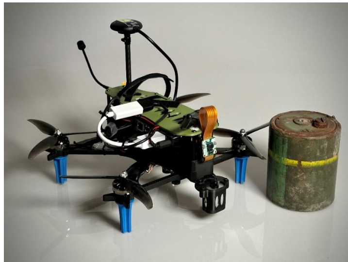
Figure 1, an FPV-drone with an example of a warhead to the right of the FPV. Photo credit: Joakim Rydell (FOI).
