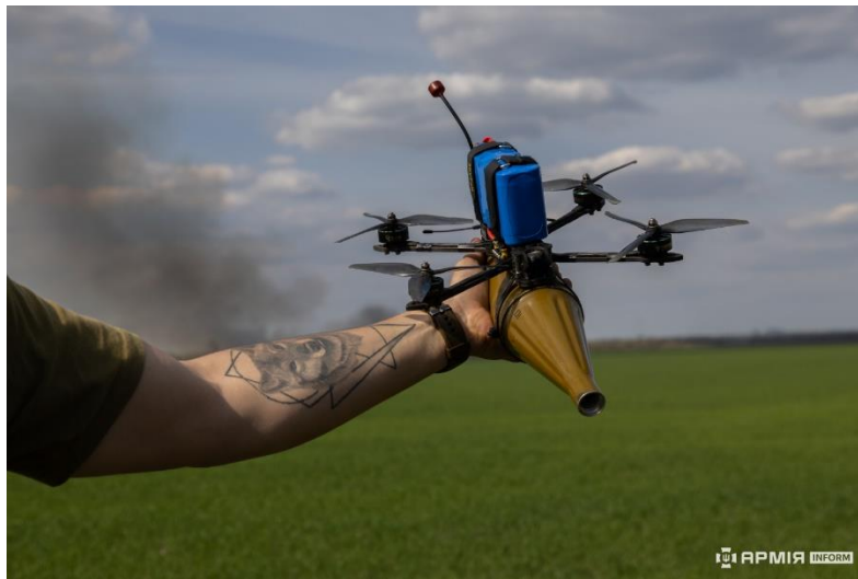
Figure 2, an example of an FPV-drone used in Ukraine. Note the anti-tank grenade mounted underneath the drone and the battery in blue strapped on top. "Ukrainian FPV loitering munition with RPG-7 ammo" by АрміяІнформ is licensed under CC BY 4.0.
