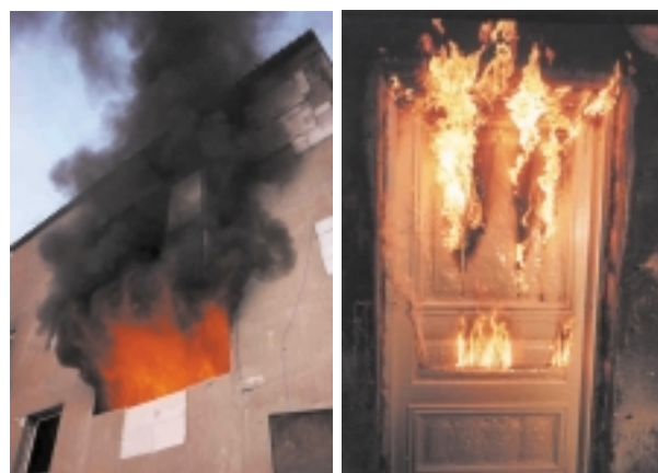
Figure 1. Full-scale fire testing of glass facades (left) and wooden panelled doors (right).
