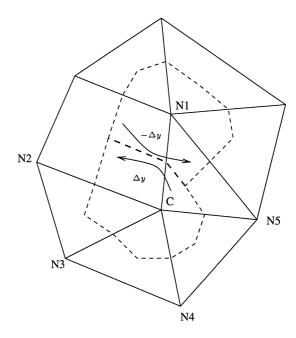
associated in a one-to-one manner with the two sides of the polygon  $\partial\Omega_C$  that have a common vertex at the side connecting the neighbour to the node C. Each neighbour will contribute to the flux with one term. This term is the mean value of  $u_C$  and  $u_{N_i}$  times  $\Delta y$  over the corresponding dual grid side. This can formally be written:
