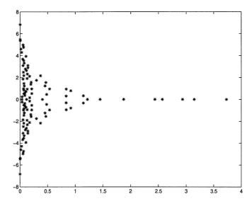
Figure 6. The spectrum of  $P^{-1}Q$  using injection, on an unstructured mesh with 105 nodes.
