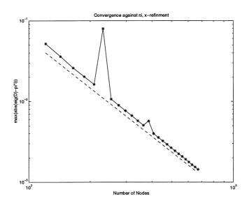
Figure 17. Convergence against the point  $2\pi i$ . New nodes are introduced in the x-direction only. The dased line is a reference line with slope -2.
