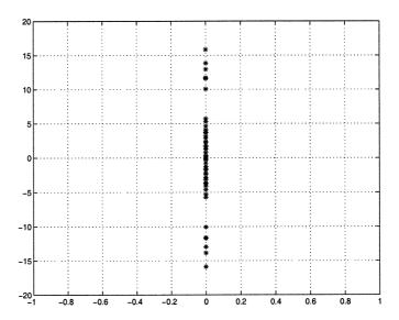
Figure 11. The eigenspectrum of  $P^{-1}Q$  with the method defined by equations (56) and (57) , computed on an unstructured mesh with 169 nodes.  $\min(\text{Re}(\lambda_i))=0$
