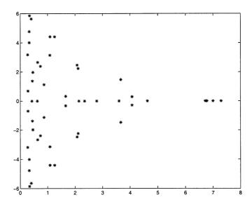
Figure 4. The spectrum of  $P^{-1}Q$  using injection, on an unstructured mesh with 49 nodes.
