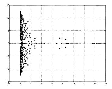
Figure 13. The spectrum of the method defined by equation (59), on an unstructured mesh with 169 nodes.  $\min(\text{Re}(\lambda_i))=0$
