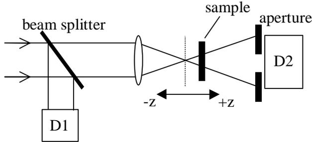
**Figure 18** Z-scan experimental set-up. The ratio of the irradiances measured by the detectors D1 and D2 is measured as a function of sample position  $z$ .
