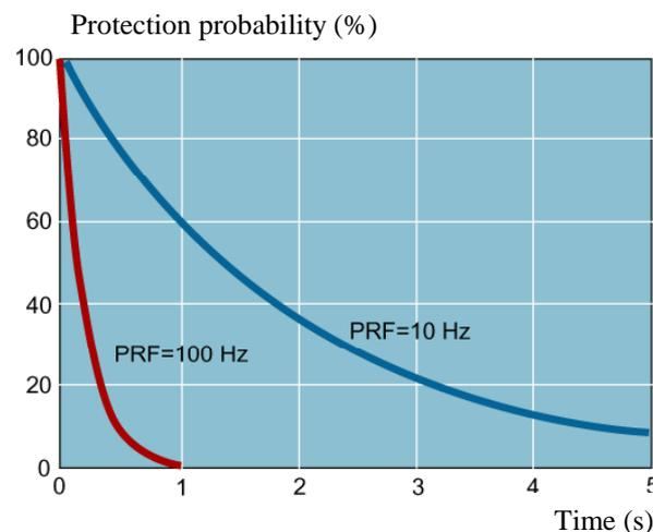
**Figure 5** The protection probability for a stochastic shutter open 5 % of the time. The laser has a pulse repetition frequency (PRF) of 10 Hz (blue curve) and 100 Hz (red line). The protection probability is quickly decreasing with increasing exposure time and increasing PRF.
