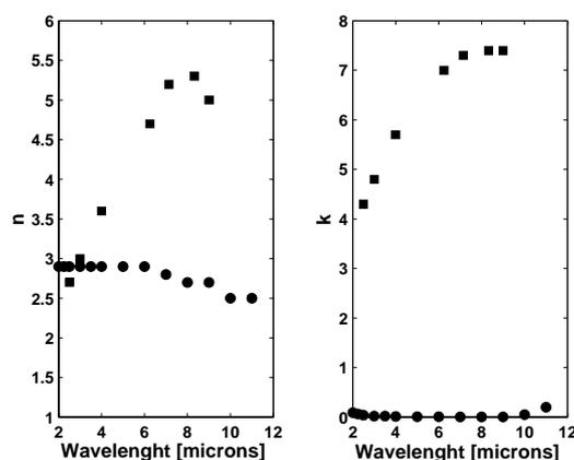
**Figure 13** Variation of the refractive index (left) and extinction coefficients (right) for the semi-conducting (circles) and metallic phases (squares) of  $\text{VO}_2$ . From ref.<sup>13</sup>
