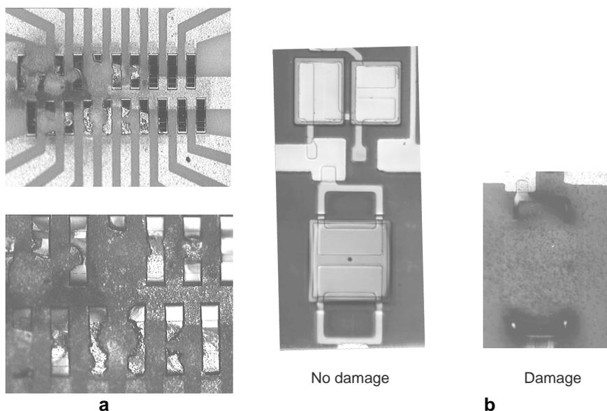
**Figure 2** Example of laser-induced damage observed in (a) HgCdTe detector and (b) Silicon microbolometer detector.
