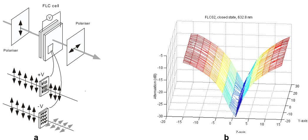
**Figure 7** a) Principle of an FLC optical shutter. b) Attenuation for an FLC-shutter as a function of the direction of the incident light.
