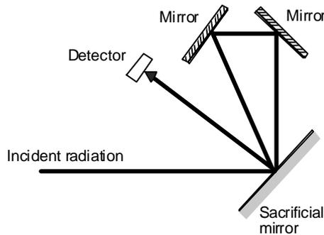
**Figure 16** Example of a sacrificial limiter in double-pass configuration using two additional mirrors.
