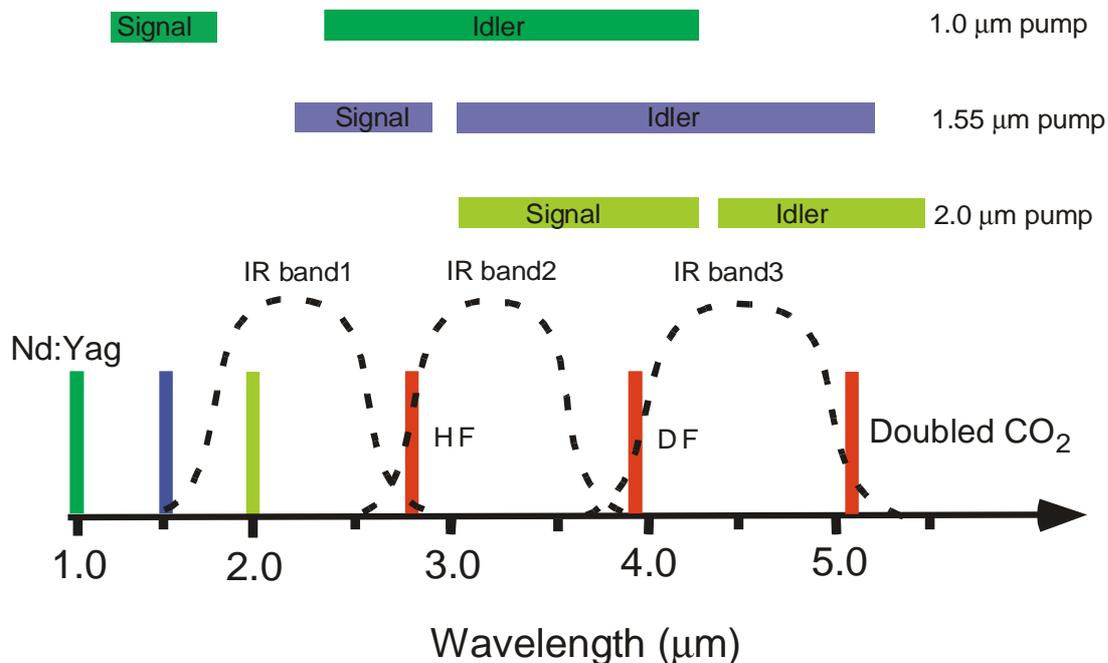
**Figure 1** Important wavelength bands for DIRCM.
