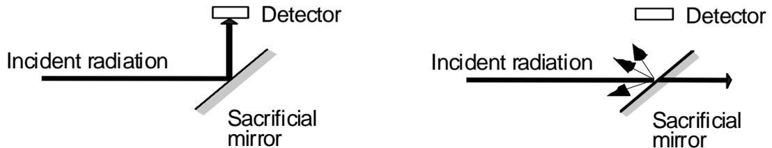
**Figure 15** The principle of a sacrificial limiter consisting of a thin sacrificial metal film on a transmissive substrate. In the operating state the mirror is reflecting the incident radiation onto the detector (left). Above the damage threshold the radiation is transmitted and partly scattered (right) protecting the detector.
