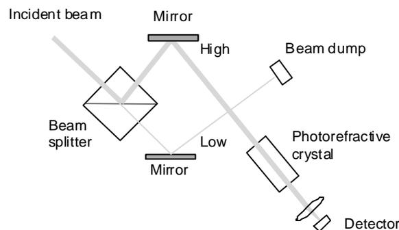
Figure 19 The principle of photo-refractive optical limiting using the beam-fanning method.
