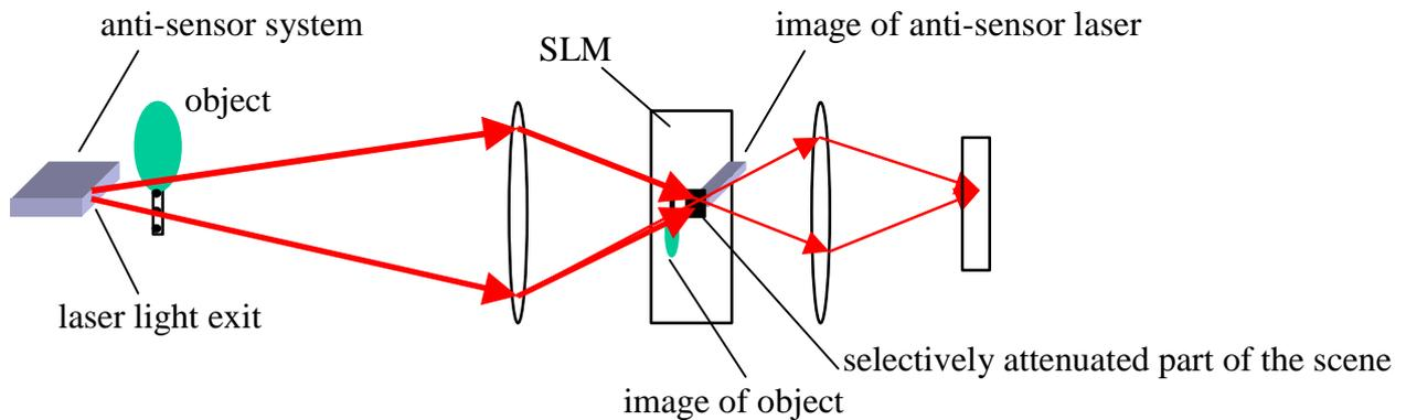
**Figure 6** Schematic illustration of an SLM positioned at a focal plane in an optical system and, thus is able to selectively attenuate radiation from parts of the field of view containing the laser light exiting an anti-sensor system.
