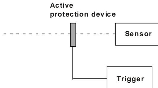
**Figure 4** The principle of active protection of EO-sensors from laser exposure.
