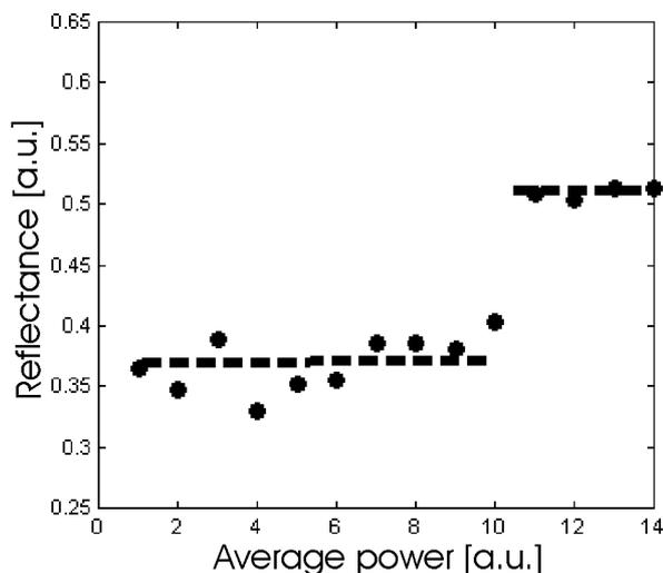
**Figure 14** Example showing switching between two states for VO<sub>2</sub> at  $\lambda = 2.8 \mu\text{m}$  which was thermally oxidised and located on a silicon substrate. The optical quality of the oxidised VO<sub>2</sub> film was rather poor in this case.
