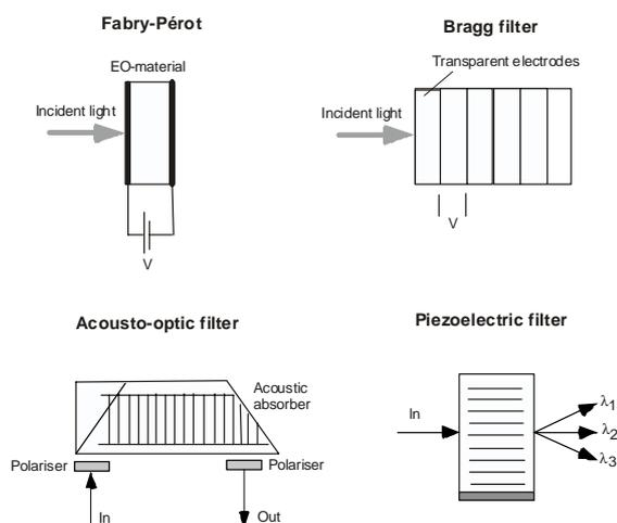
**Figure 9** Example of methods for tuneable filters.<sup>4</sup>
