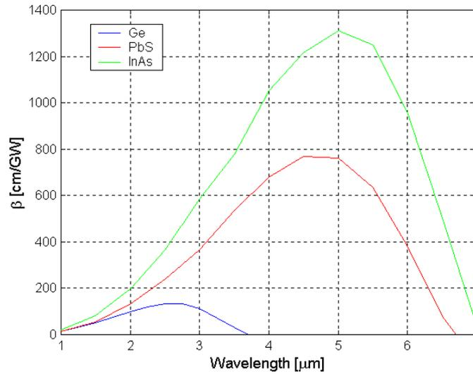
**Figure 11** The two-photon absorption coefficient as a function of  $\lambda$  for Ge, PbS and InAs.
