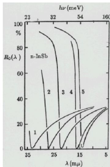
**Figure 20** Reflection spectrum of n-type InSb with the different electron densities  $3.5 \times 10^{17}$ ,  $6.5 \times 10^{17}$ ,  $1.2 \times 10^{18}$ ,  $2.8 \times 10^{18}$  and  $4 \times 10^{18} \text{ cm}^{-3}$ , for curves 1-5, respectively [W.G. Spitzer and H.Y. Fan, Phys. Rev. 106, 882 (1957)].
