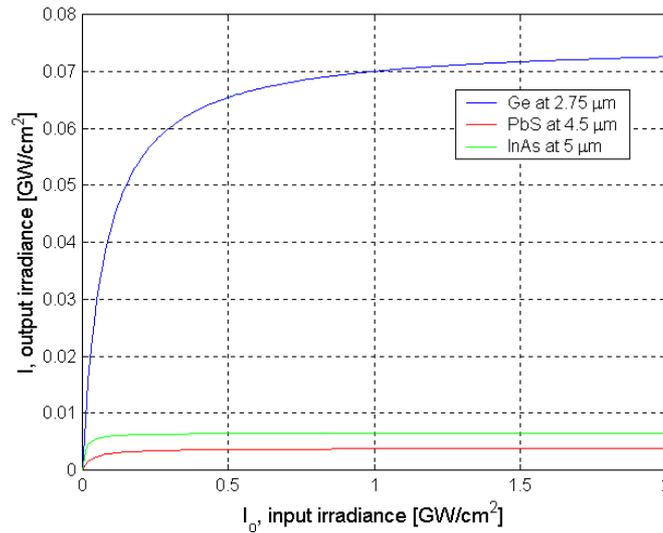
**Figure 12** The input and output irradiance for Ge, PbS and InAs at 2.75, 4.5 and 5μm, respectively, calculated using Eq. (7)
