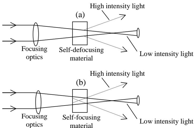
**Figure 17** The concepts of self-defocusing (a) and self-focusing (b).
