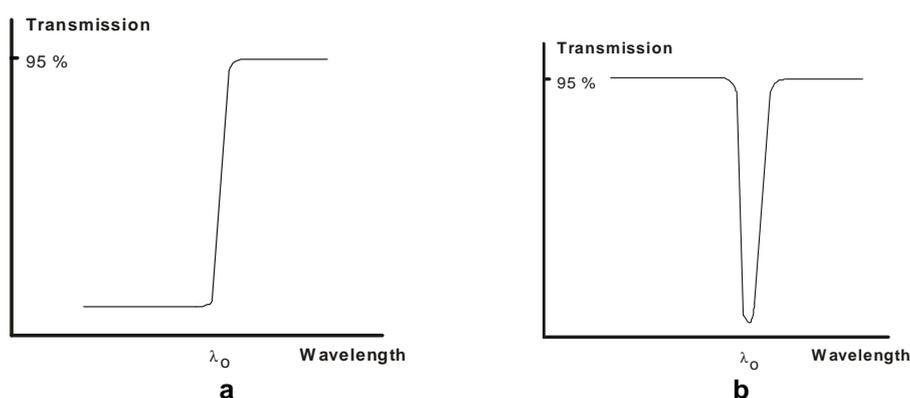
**Figure 3** Characteristics of a low-pass (a) and notch filter (b).
