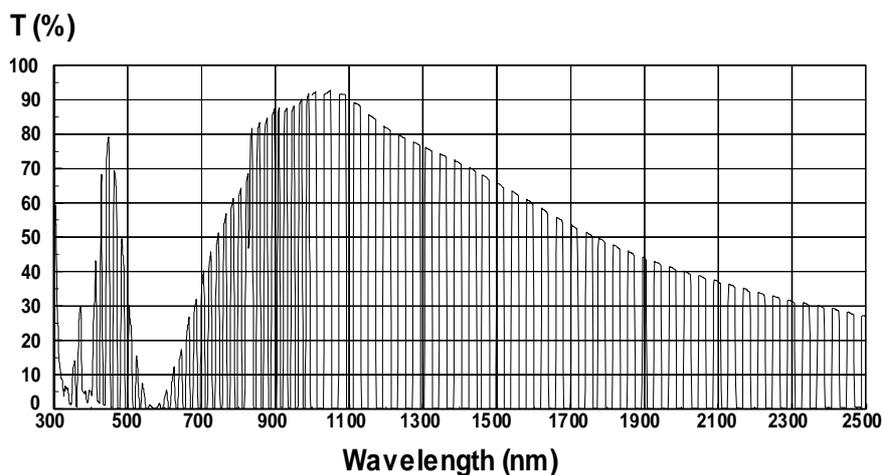
**Figure 8** Transmission of a standard commercial FLC material in a 4 μm thick cell.
