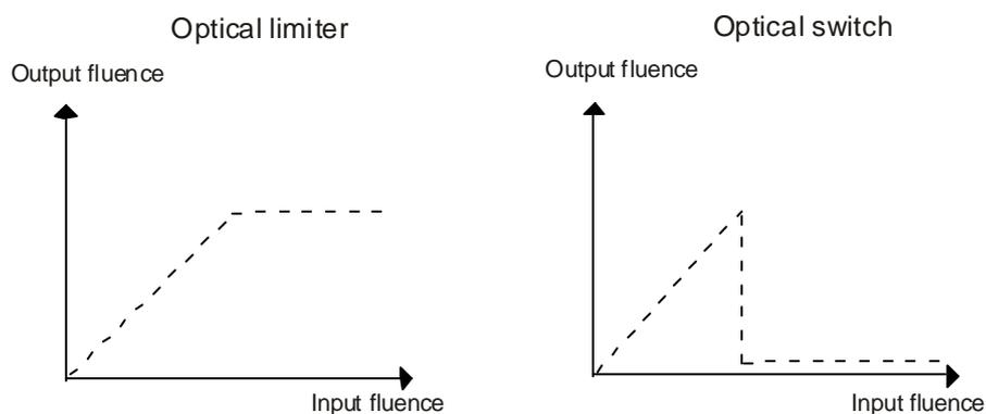
**Figure 10** Schematic behaviour of self-activating protection devices.
