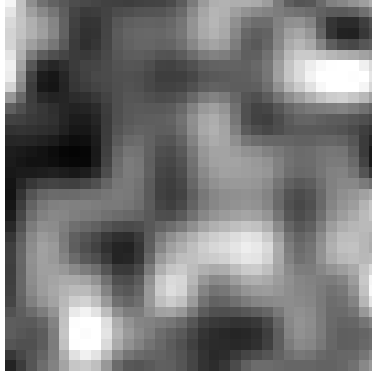
Figure 2.10. One pixel with turbulence cells of a specific cell size and random values determined by the turbulence pdf, equation (2.13). White represents a higher intensity than black.
