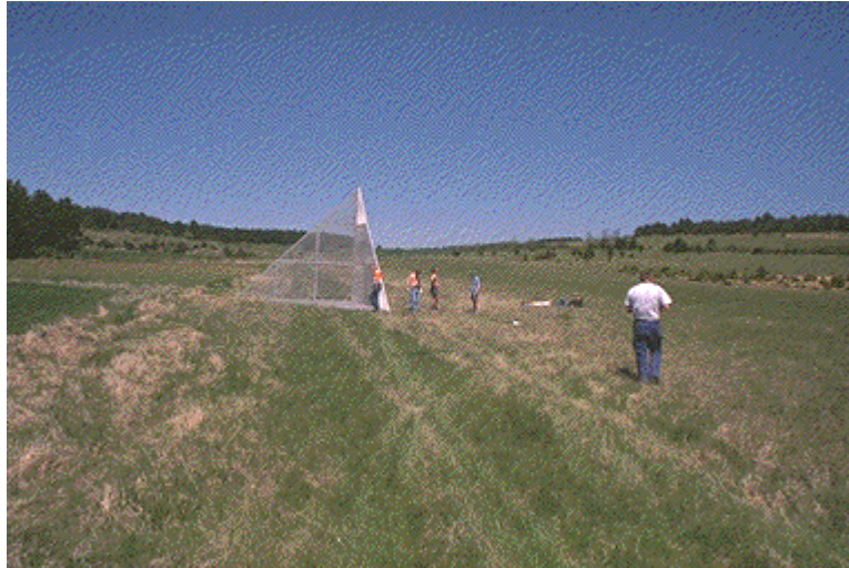
Figure 30. Trihedral FOA-T3 deployed on the grass close to the airfield.
