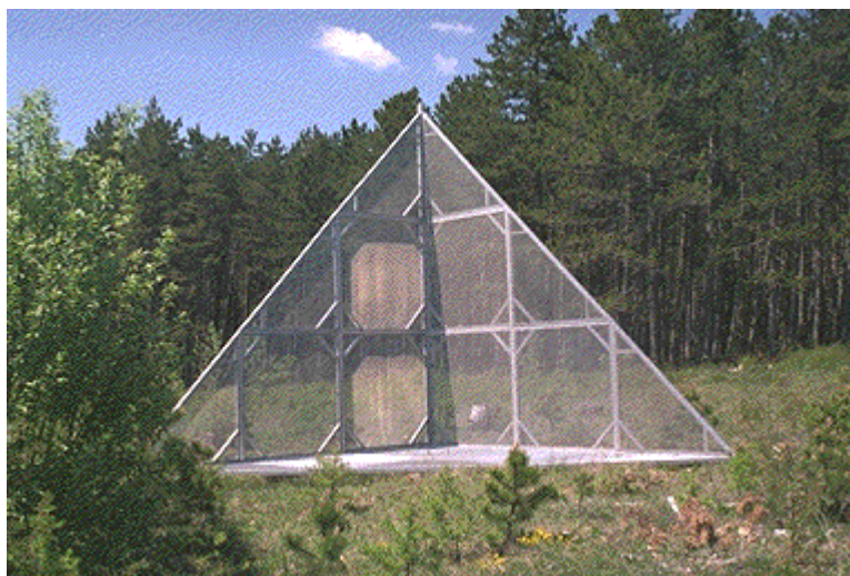
Figure 29. Trihedral FOA-T2 deployed in a clear-cut area.
