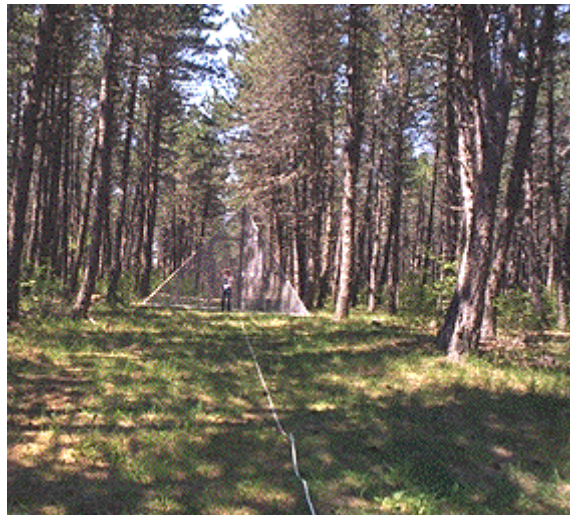
Figure 28. Trihedral FOA-T1 deployed along narrow clearing between stands #277 and #278.
