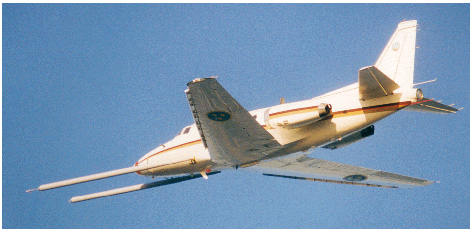
Figure 1. The Sabreliner aircraft, owned and operated by FMV:Prov, with the antenna system for CARABAS-II installed. (Courtesy: FMV:Prov).
