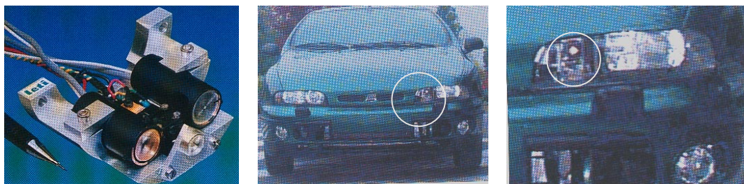
Figure 96. Example of very compact laser radar using a 1.5\ \mu\text{m} \mu\text{chip} laser for use on cars. From Leti France.
