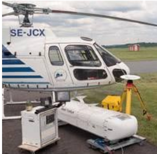
Figure 66. The TopEye system comprises a pod with the laser rangefinder, an on-board computer and a GPS ground reference station.
