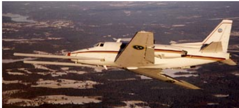
Figure 88. The Sabreliner aircraft with the broadband CARABAS-II VHF push boom antenna arrangement. (Courtesy: FMV:Prov).
