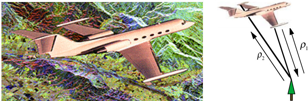
Figure 83. Artist's impression of the GeoSAR realization onboard a Gulfstream II, cruising over a fairly hilly landscape with forested regions (left). The selected platform will give the system an area coverage rate of about 4 km 2 /s. The X-band antennas are mounted under the fuselage, whereas the P-band antennas are located within pods affixed to the ends of the wings to create a 20 m interferometric baseline (right). From http://southport.jpl.nasa.gov/html/projects/geosar.html .
