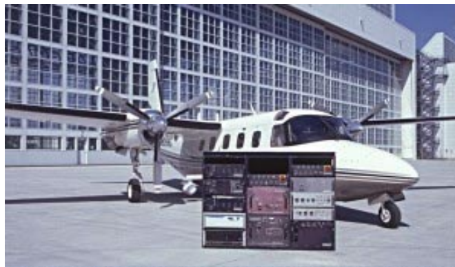
Figure 86. The AeS-1 aircraft with the radar electronics as an inset in the middle. One of the three X-band antennas affixed to a rigid boom is barely visible just to the left of the hardware section. ( http://www.aerosensing.de ).
