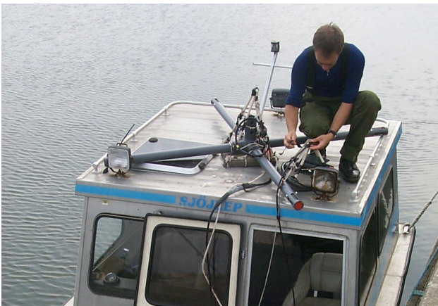
Figure 4. The 2-axis electrode sensor is the cross. The smaller Bartington fluxgate magnetometer is here under preparation.
