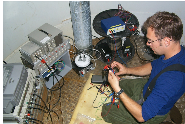
Figure 5. The registrations of the electrical and magnetic field were performed from the inside of the mill tower.
