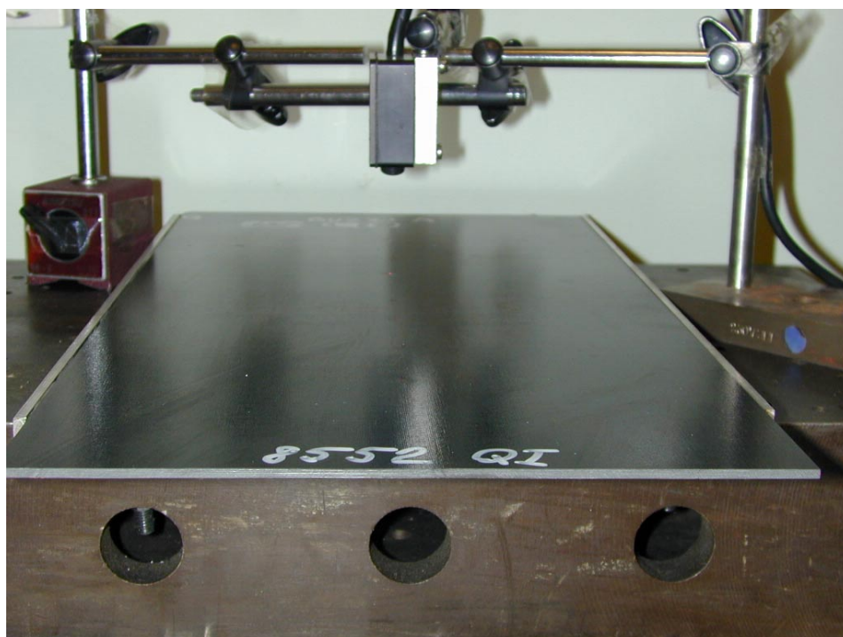
Figure 4 Set-up for measurement of dent depth
