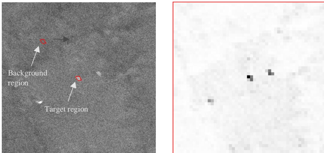
**Figure 9** When the background region is set to be identical in shape and size to the target region then the GLCM technique can be used to identify target like objects in the image.
