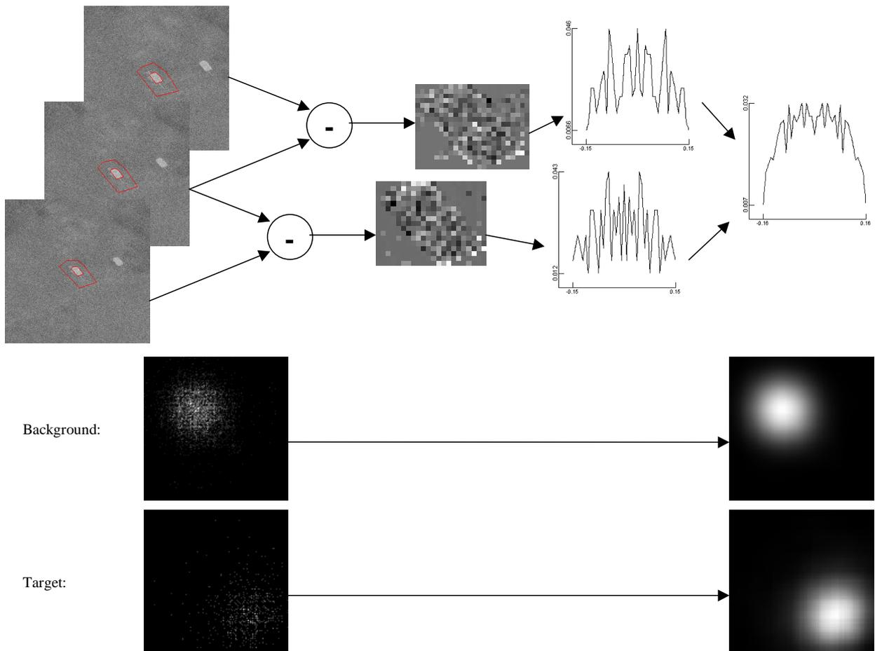
**Figure 4** The uncertainty in target pixel intensities is used to blur the GLCMs of the target and background (both GLCMs are blurred by the same uncertainty histogram). Only pixels on the target are used to determine the shape of the uncertainty histogram.
