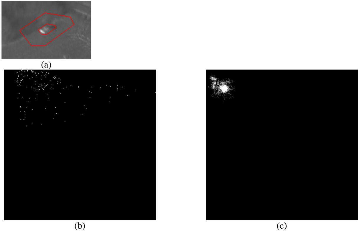
**Figure 3** (a) Image with target area and background area enclosed with red lines. The target region is the inner region and the background area is the outer region. The background and target areas have no pixels in common. (b) GLCM of the target region. (c) GLCM of the background region.
