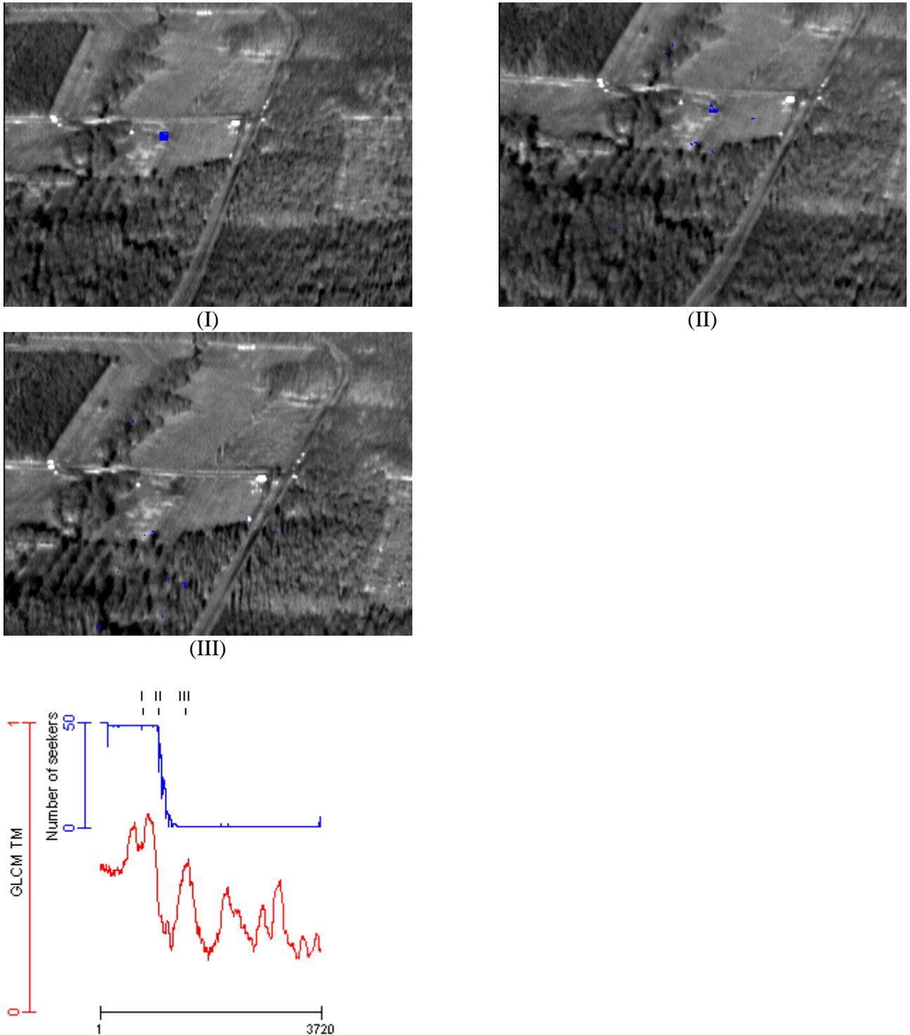
**Figure 14** GLCM TM calculation for a sequence where MWF is used to conceal one of two armored vehicles. The red curve show the maximum GLCM TM result for the concealed vehicle and the blue curve is the result from tracking the concealed vehicle using a correlation tracker (number of seekers within 10 pixels from the target). The blue pixels in the images from the sequence show the positions of the 49 different correlation trackers.
