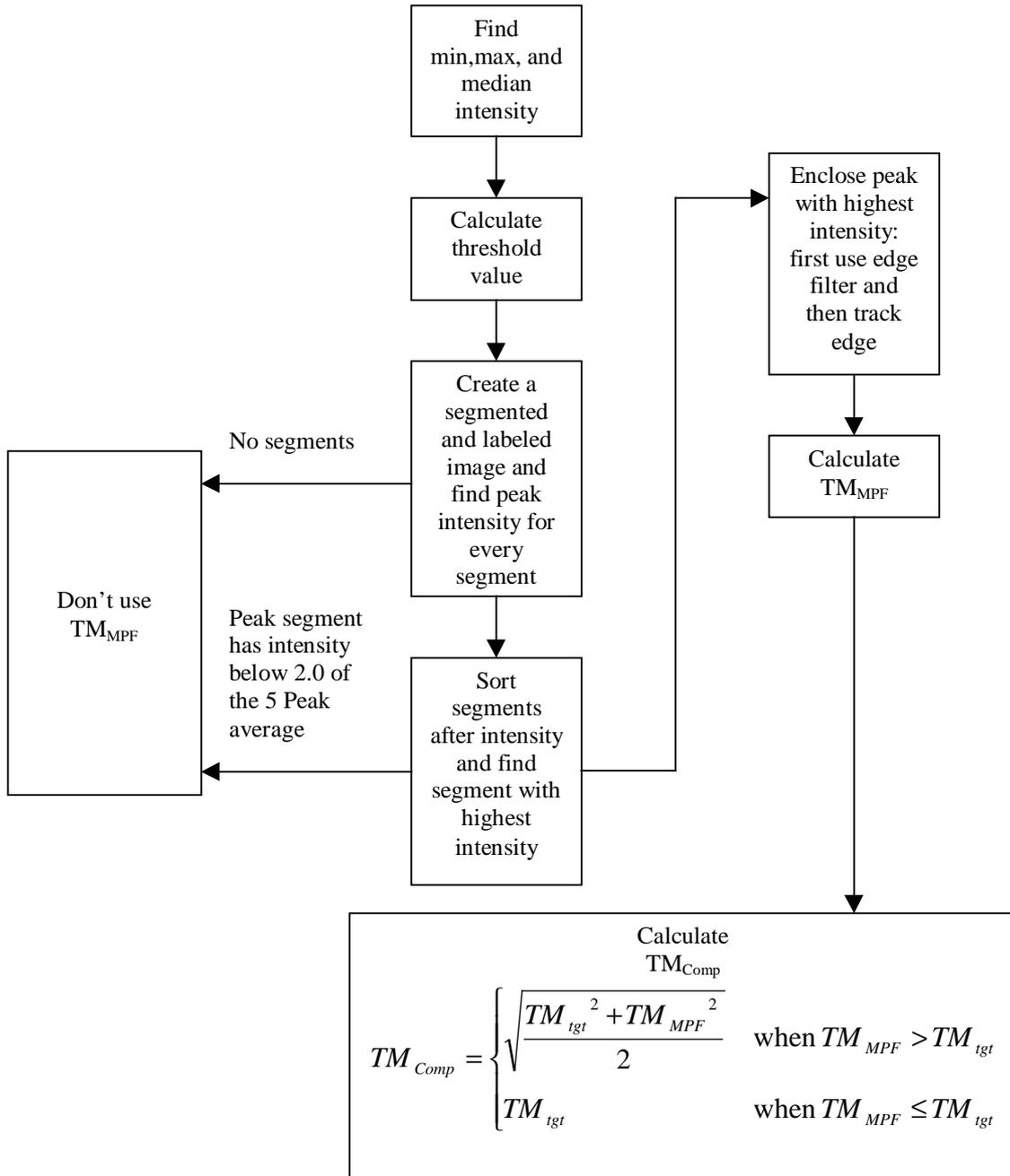
**Figure 7** Flow chart when the GLCM TM is calculated for targets with a predominant feature (e.g. a hot spot)
