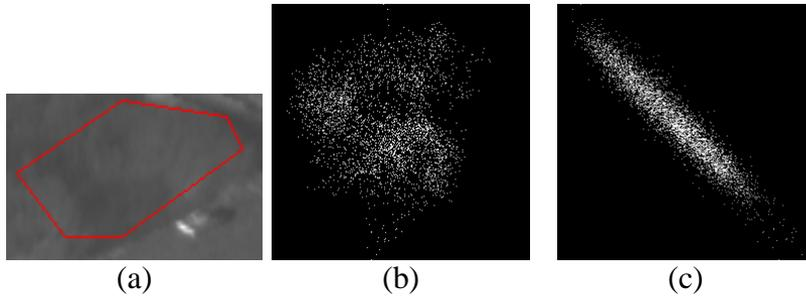
**Figure 1** (a) Image where the area for GLCM calculation is enclosed (red), (b) GLCM with large displacement (20 pixels), (c) GLCM with small displacement (1 pixel).
