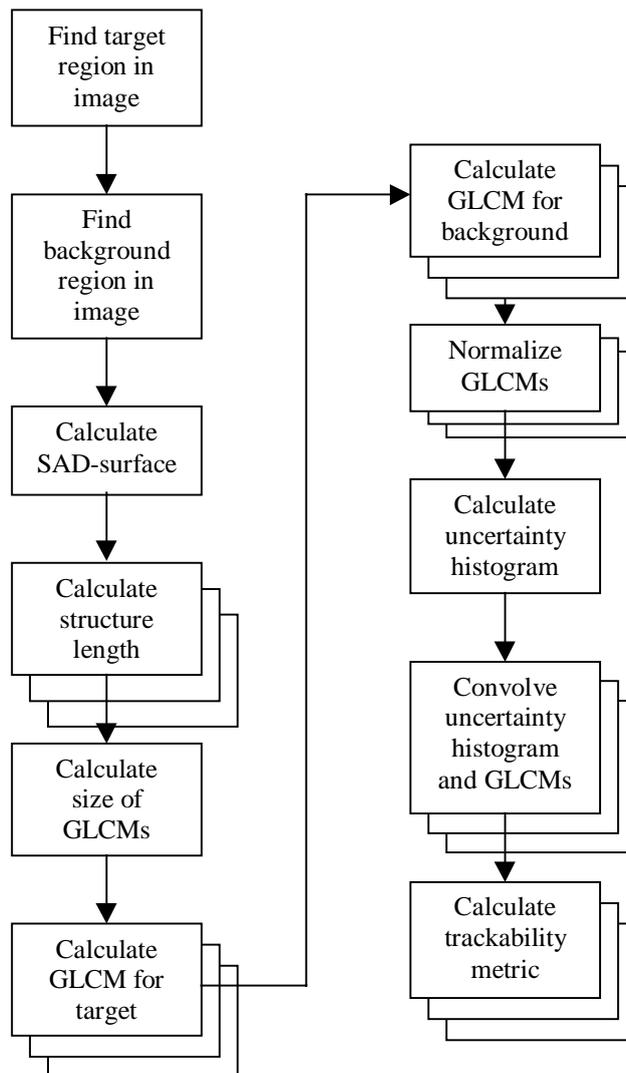
**Figure 6** Flow-chart when the GLCM trackability metric is calculated. A box in the foreground of other boxes indicates that more than one direction can be used.
