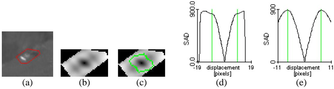
**Figure 2** (a) Image with target area enclosed with a red line. (b) SAD surface, (c) SAD surface showing the target's structure length for different directions (in green). (d) Horizontal cross-section of SAD surface showing the position of the target's structure length. (e) Same as in (d) but with a vertical cross-section.
