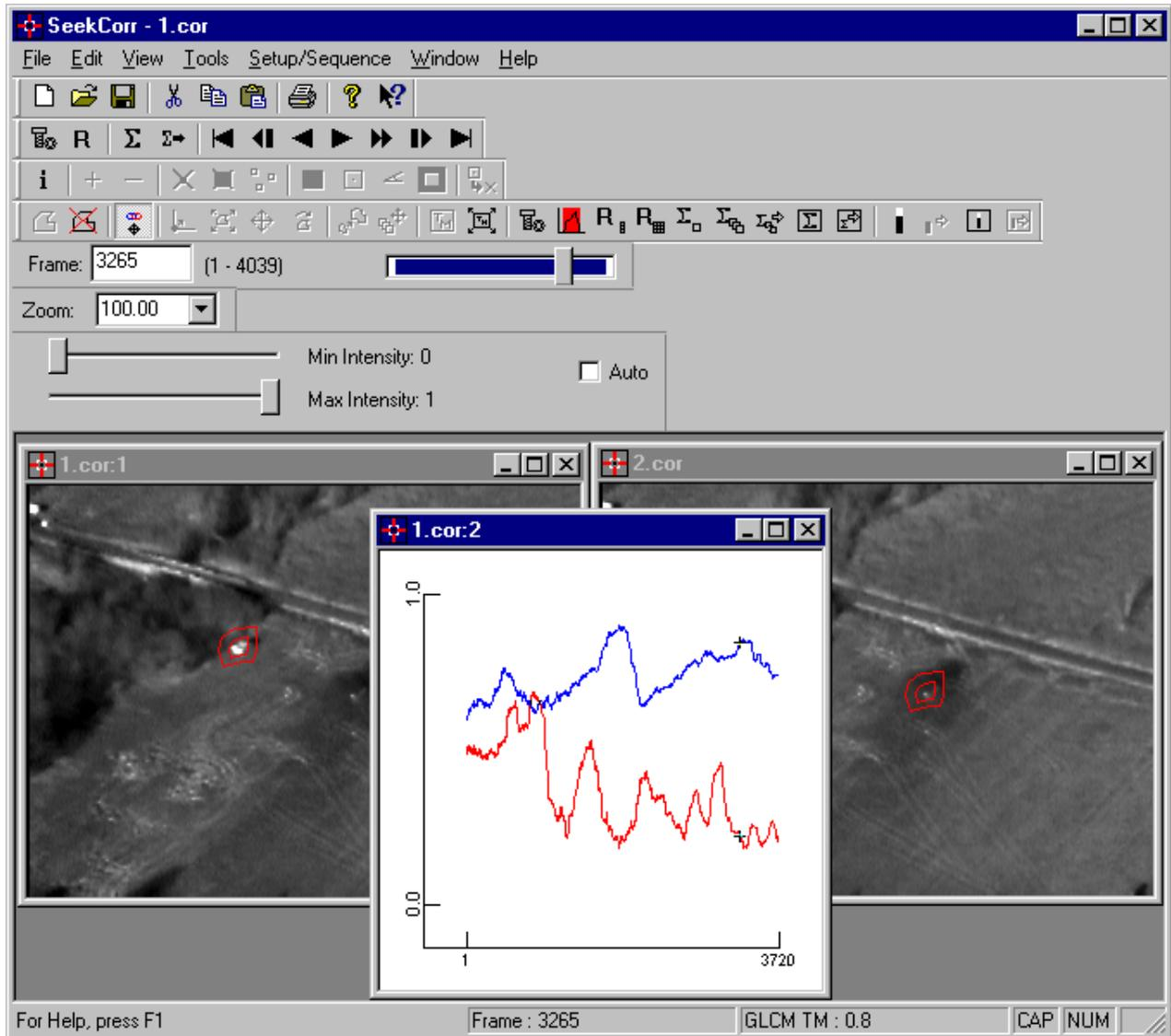
*Figure 11 Graphical user interface of the program for GLCM TM calculations.*
