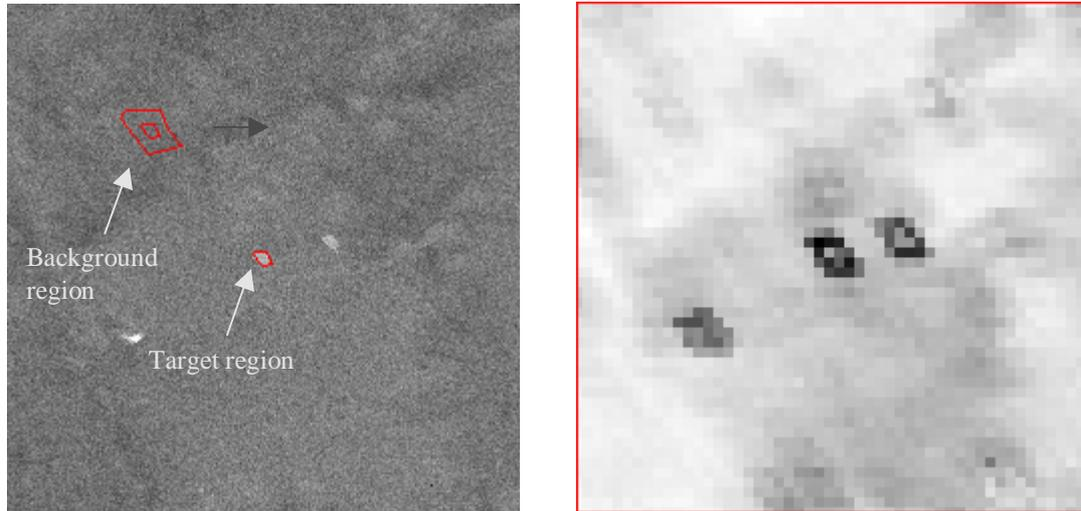
**Figure 8** Image to the left and the result of a GLCM TM calculation for the whole image to the right. In this type of calculation the target region is kept at a fixed position while the background region moves across the image.
