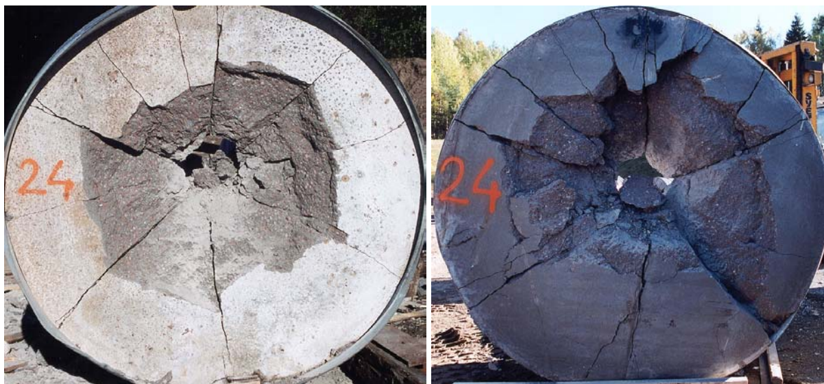
Figure 4.5. Target after perforation for test no. 24, front face to the left
