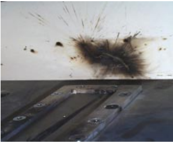
Figure 2: Cardboard with splash and burn marks of transversely accelerated rod in EM armour experiment. Note the trace of rod and current arc along the lower armour plate. Upper plate is removed.
