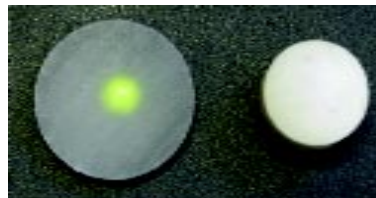
Figure 4. Al_2O_3 samples. The left sample shows an example of an opaque Al_2O_3 produced by SPS (the grain size is in the same order as the wavelength of light, 400-700 nm), with a green light diode behind, and the right sample a traditionally sintered Al_2O_3 .
