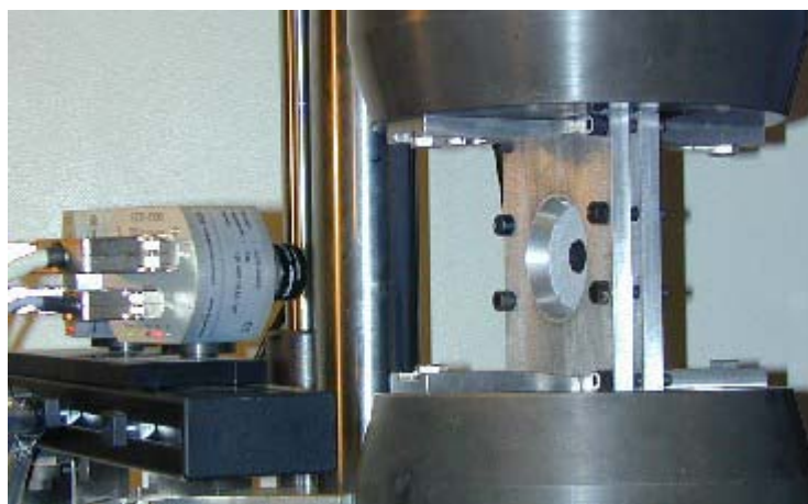
Figure 4.4 Anti-buckling support on a 100 mm width specimen.
