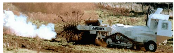
Example of Mechanical Demining Equipment - the Aardvark™
