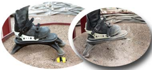
"Spider Boot" evaluated against an AP mine (97g)
