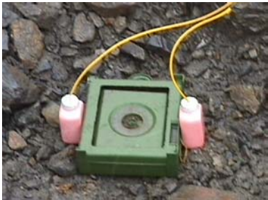
FIXOR™ positioned to destroy an AT mine
