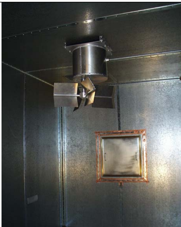
Figure A2. The small stirrer in the 37 m 3 chamber E3. Rotational volume 0.11 m 3
