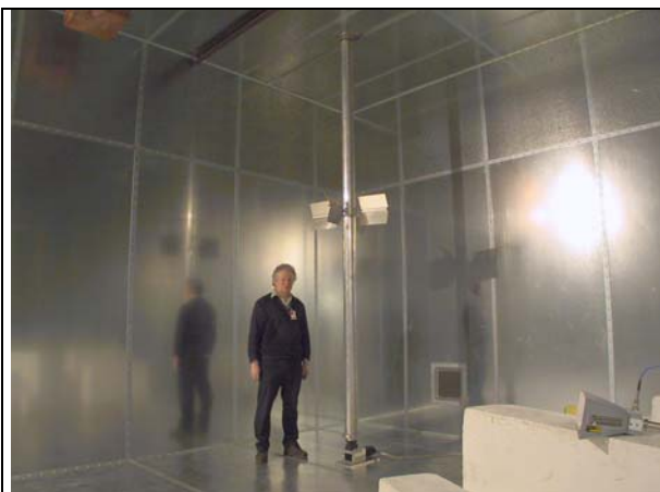
Figure A11. The small stirrer in the 210 m 3 chamber at Bofors. Stirrer Rotational volume 0.11 m 3
