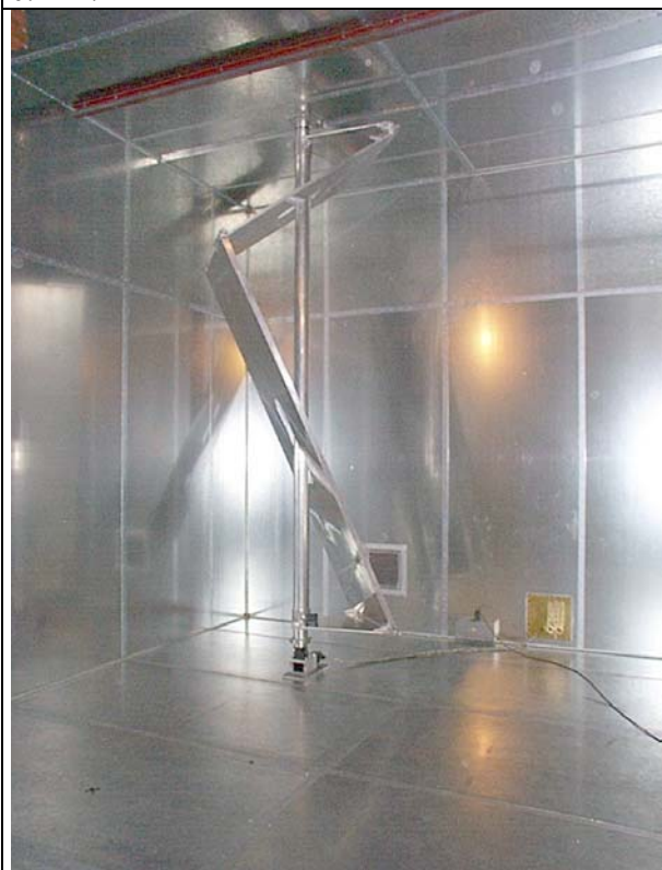
Figure A13. The original stirrer in the 210 m 3 chamber at Bofors. Rotational volume 4 m 3 .
