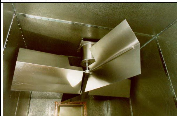
Figure A3. The large stirrer in the 37 m 3 chamber E3. Rotational volume 3.93 m 3
