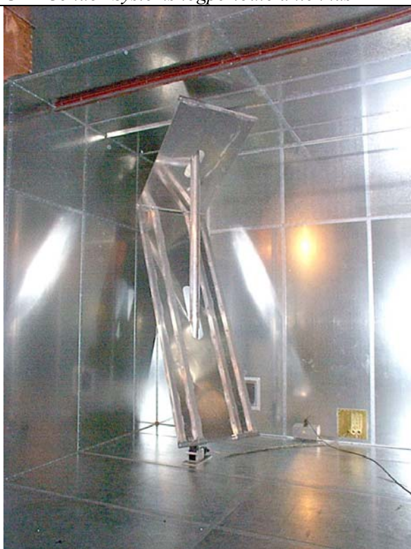
Figure A14. The original stirrer in the 210 m 3 chamber at Bofors. Rotational volume 4 m 3 . Tuner in other position.
