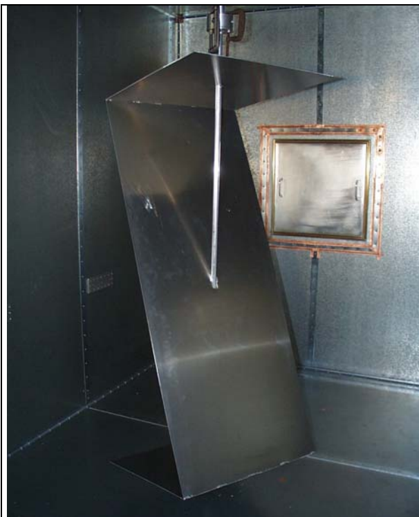
Figure A1. The long stirrer in the 37 m 3 chamber E3. Rotational volume 0.88 m 3
