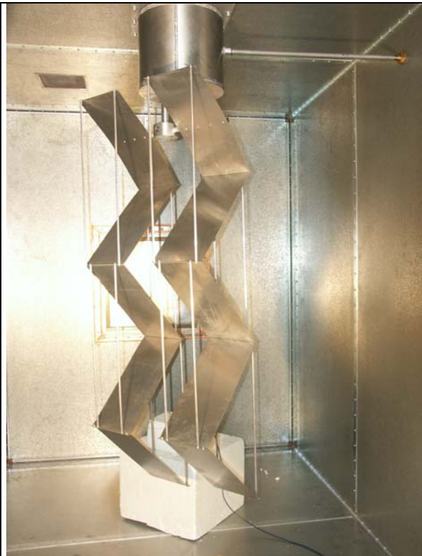
Figure A5. The improved long stirrer in the 37 m 3 chamber E3. Rotational volume 0.88 m 3
