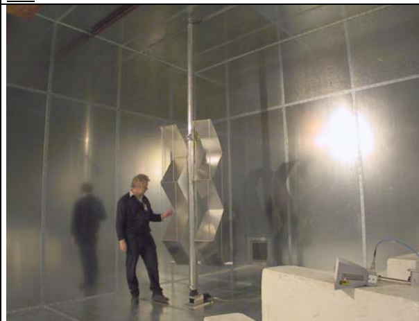
Figure A9. Bofors 210 m 3 Chamber. The improved long stirrer . Rotational volume 0.88 m 3 .
