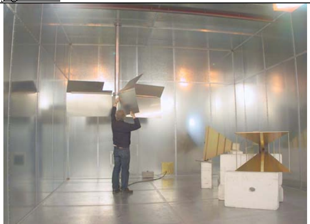
Figure A10. The large stirrer in the 210 m 3 chamber at Bofors. Rotational volume 3.93 m 3
