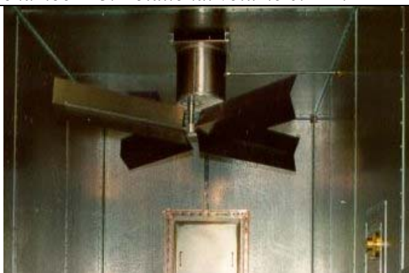
Figure A4. The basic stirrer in the 37 m 3 chamber E3. Stirrer rotational volume 1.18 m 3
