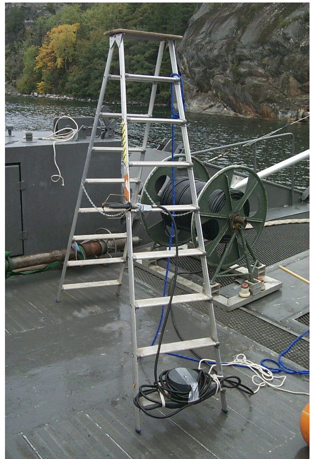
Figure 3.4: The step target with a monitor hydrophone.
