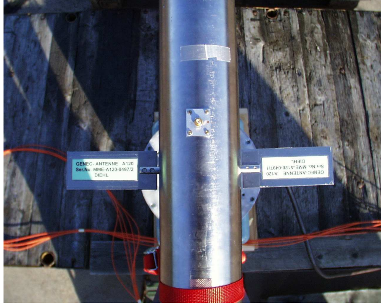
Figure 3.5: GENEC on top of the turntable. GENEC does here rotate in the wing plane. During all RS-test GENEC was positioned on the turntable as in this figure.
