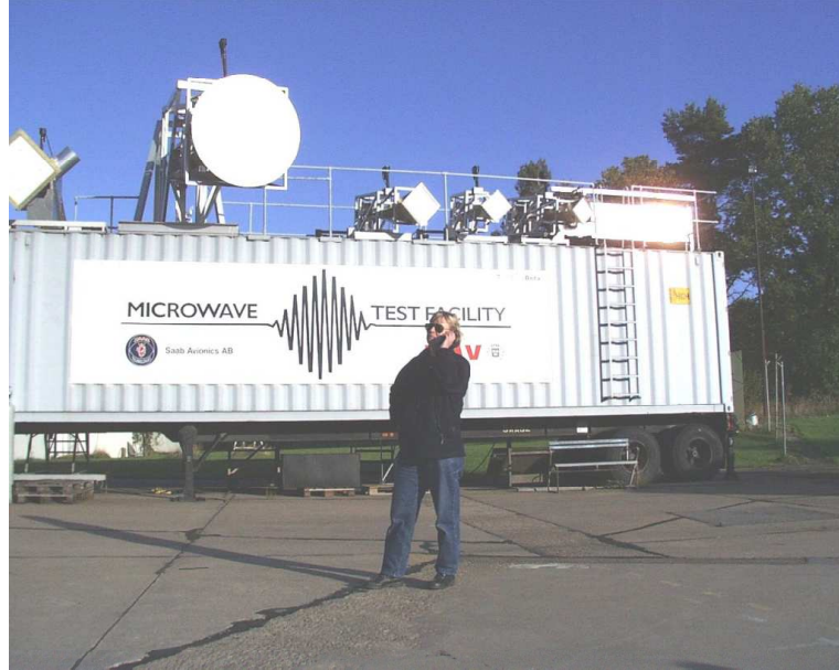
Figure 3.3: The Microwave Test Facility (MTF). On top of the MTF the S-band (2.857 GHz), the L-band (1.300 GHz), the C-band (5.710 GHz), the X-band (9.300 GHz) and the Ku-band (15.00 GHz) antenna, respectively, can be seen.
