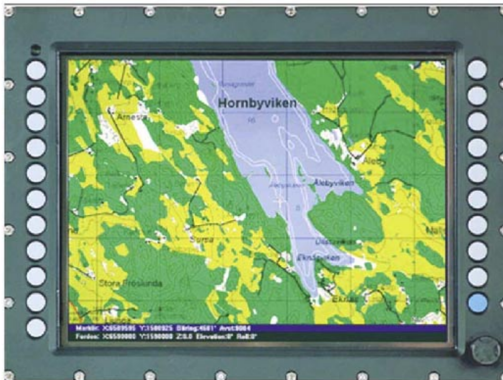
Bild 2 Vehicle command and control system (VCCS)
