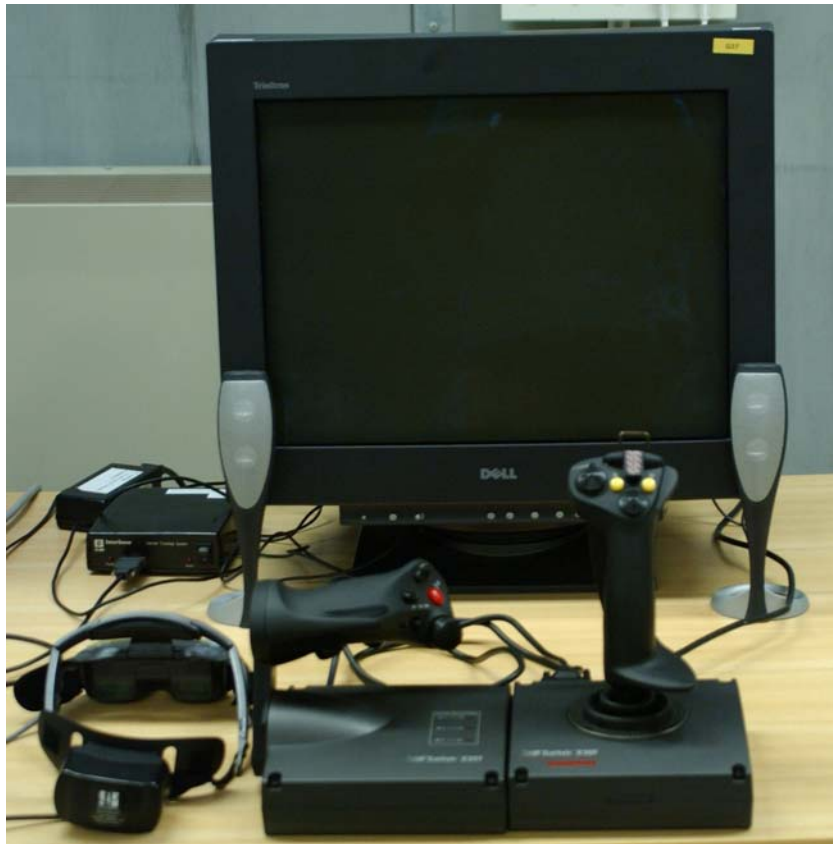
Figure 4. Pilot station with VR-goggles including head tracker, Saitek throttles and flight control sticks, sound system and a monitor presenting the instrumentation.
