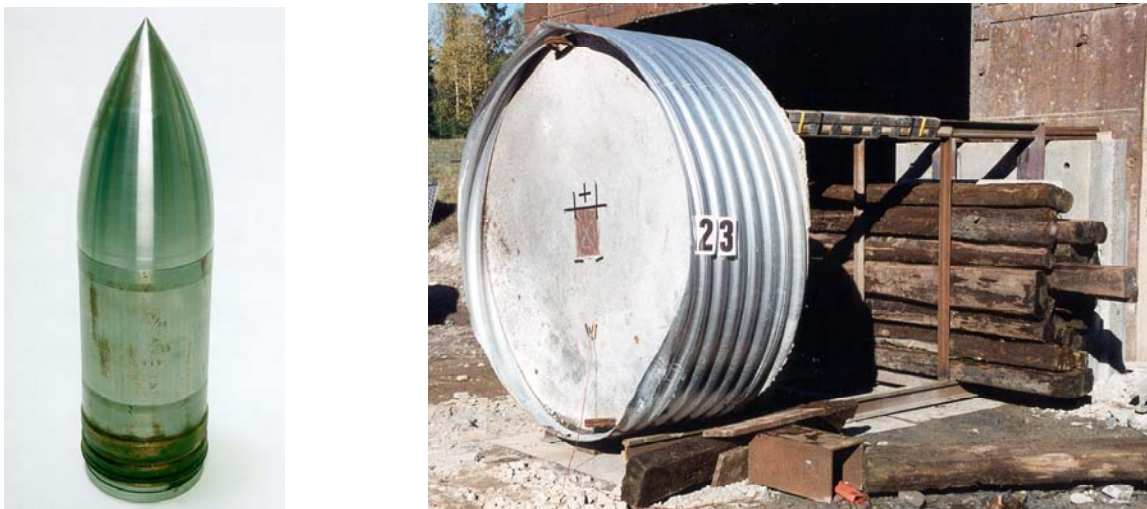
Figure 3.1. The steel projectile and the concrete target used for the benchmark tests in 1999, see also appendix 2. From Hansson 2001.
