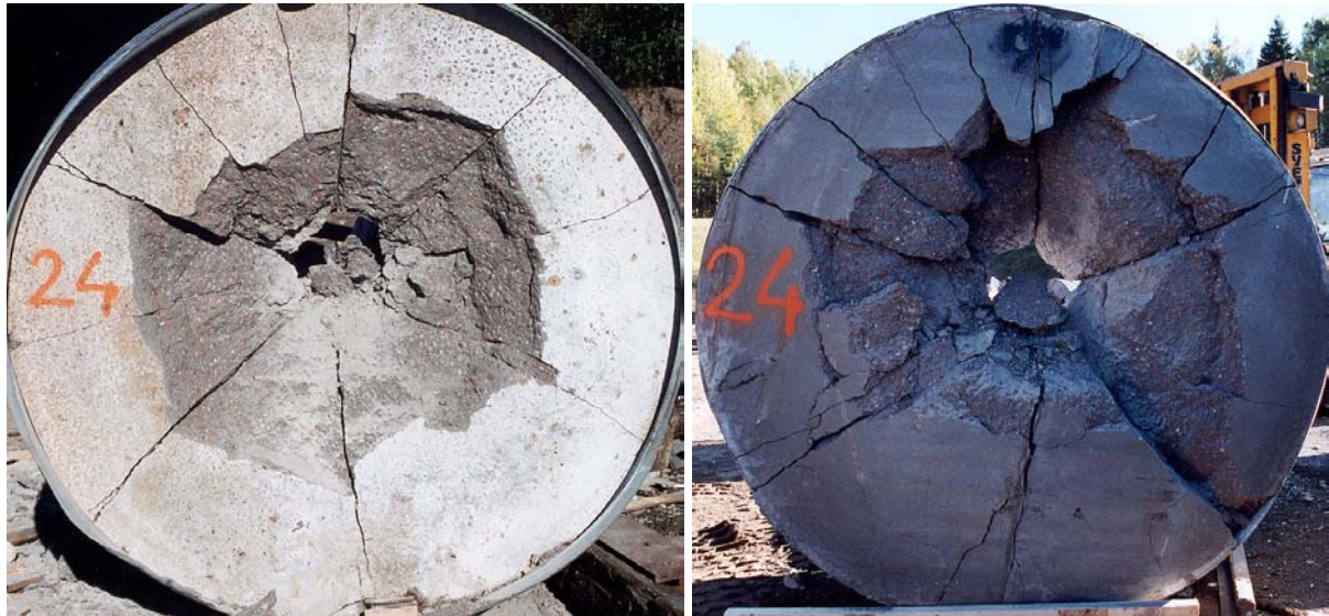
Figure A.2.9. Target after perforation for test no. 24, front face to the left.
