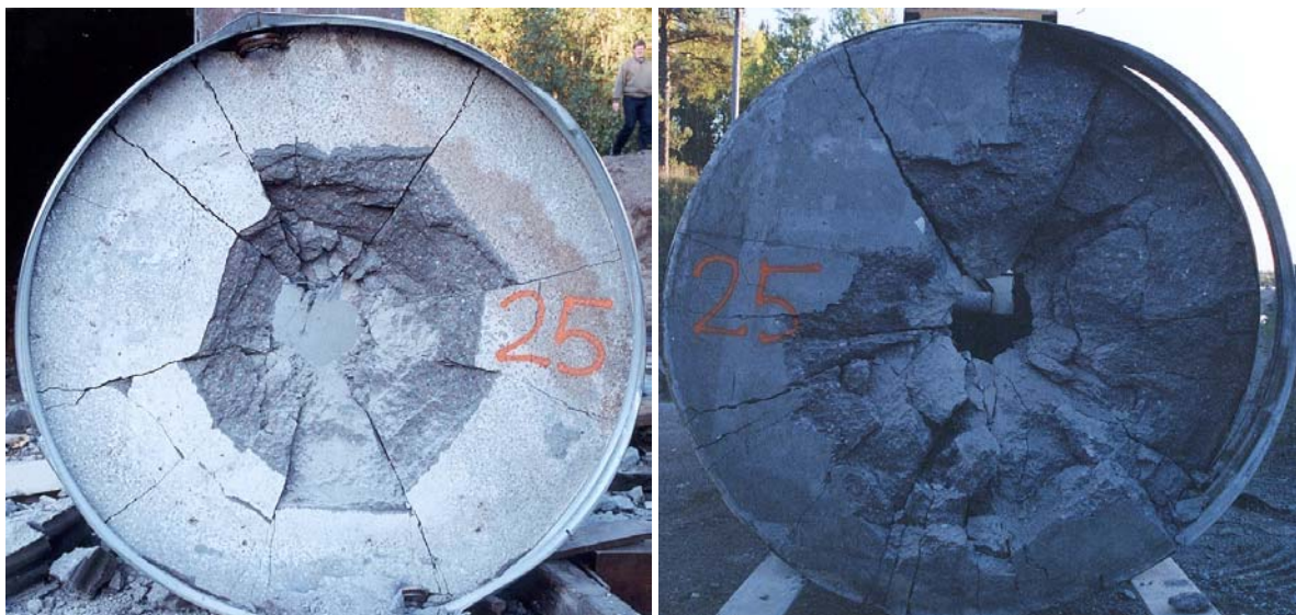
Figure A.2.10. Target after perforation for test no. 25, front face to the left.
