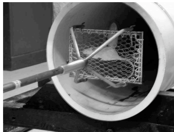
Fig. 2. The tire netting cage for fixation of rat during blast exposure
