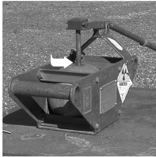
Fig 6. The Co-60 source elevated to radiation position. The source is mounted at the bottom of the vertical rod. The white arrow points to the source position.
