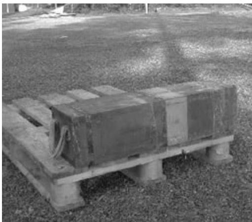
Fig 7. Blind ammunition box of wood filled with concrete. A large number of these boxes were used for shielding of the sources during the exercise. The outer dimensions are 720 \times 185 \times 200 mm and the wood is 22 mm thick.
