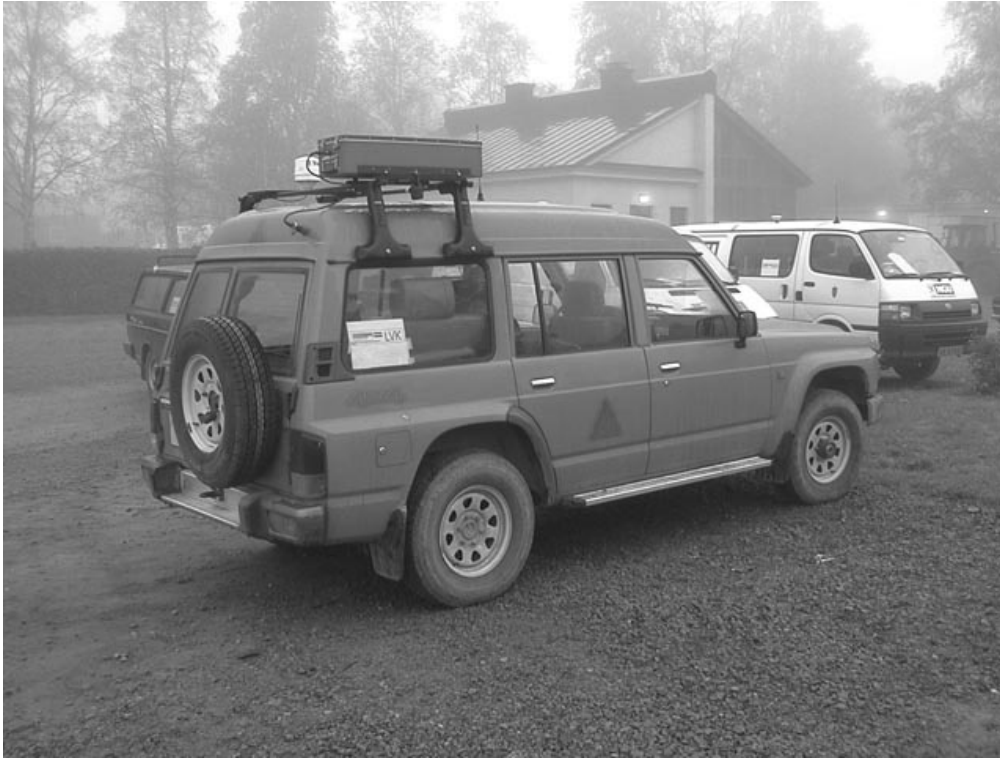
Fig 18. The car of the Latvian CGS team LVK from the Lielrigas Regional Environmental Board, Radiation Safety center. Measuring equipment was a 4 litre sodium iodide detector from Exploranium mounted on the top of the car. Positioning was made by a differential geopositioning system (DGPS). Measurements data were transferred to a laptop computer and processed using Nucspec v.2.1 and Mapinfo software.
