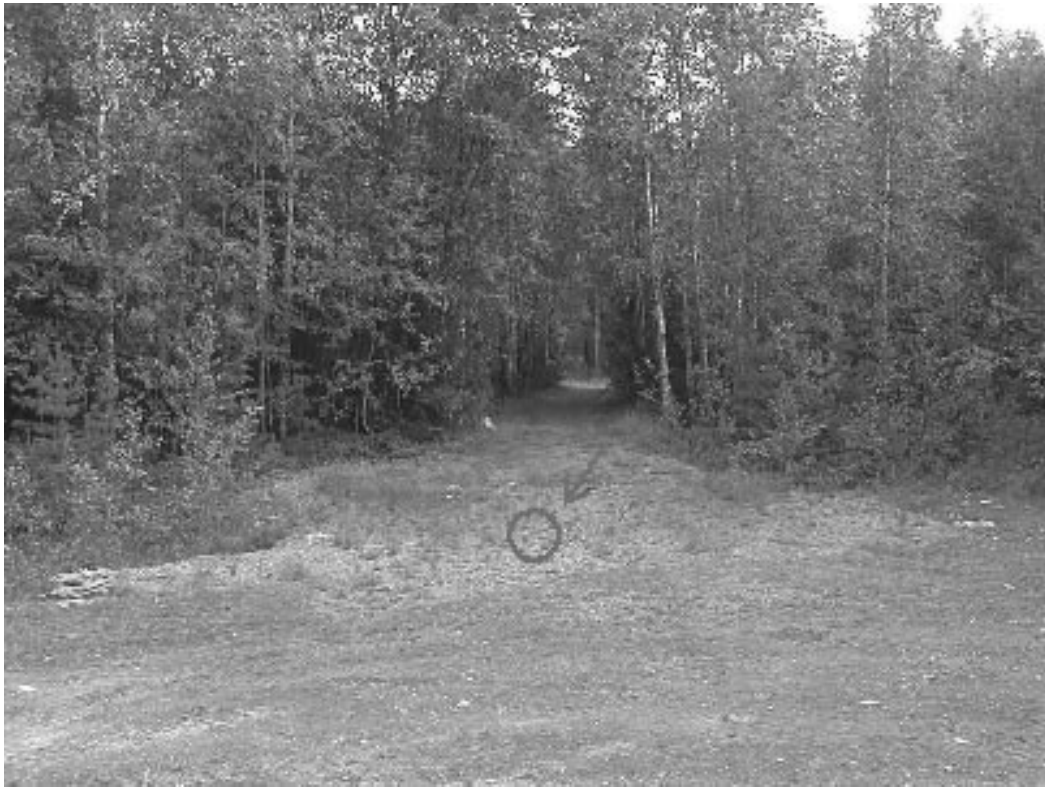
Fig 14. The strongest Co-60 source of 40 GBq (5:1) was a radiographic source placed in a drainage drum at a depth about 50 cm under a road in area A5. The source position under the road is indicated in the picture with a ring.
