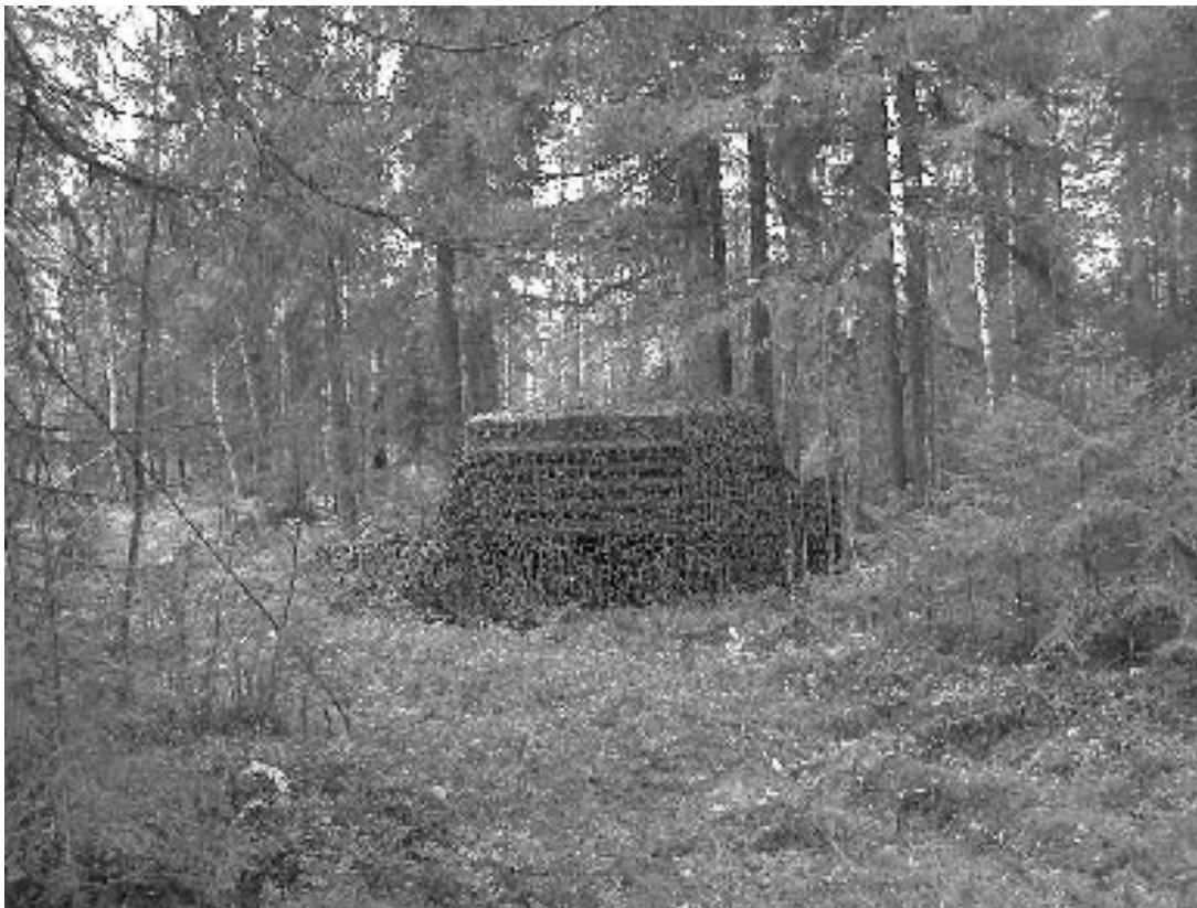
Fig 13. Some sources were placed in tracked vehicle carts. The picture shows the masked cart of source 2:3 containing an opened hospital Mo-99 - Tc-99m generator of 0.7 GBq. The source was collimated upwards and never detected, nor by airborne or car-borne teams.
