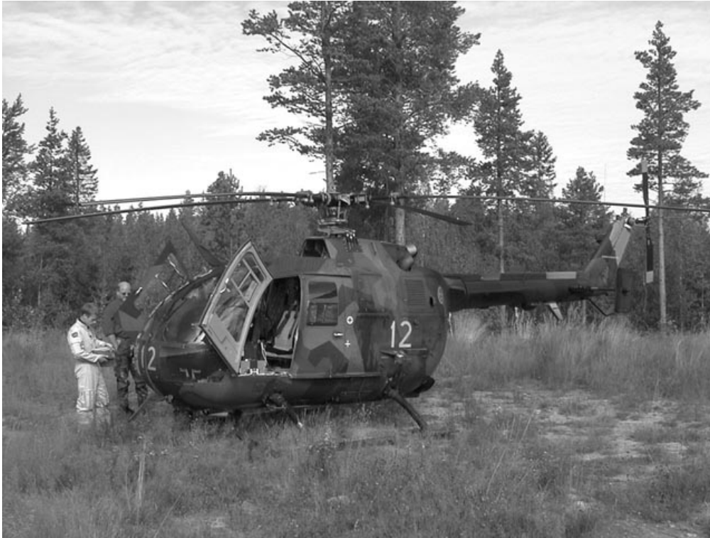
Fig 16. The Swedish army helicopter HKP-9 (MBB BO 105) used by the Swedish AGS teams SEB from the Swedish Radiation Protection Authority and SEC from the Swedish Defence Research Agency. The measuring equipment of team SEB was a 5"x 5" sodium iodide detector (1.6 litres) with a GDM 40 RPS analyzer and a 70 % high purity germanium detector with a Dart analyzer.
