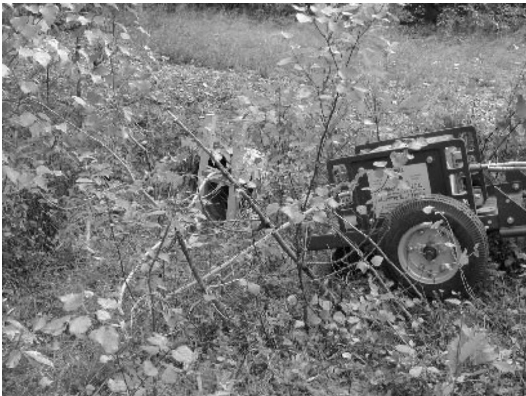
Fig 15. The road drum, the source guide and the transport container for the radiographic Co-60 source in area A5.
