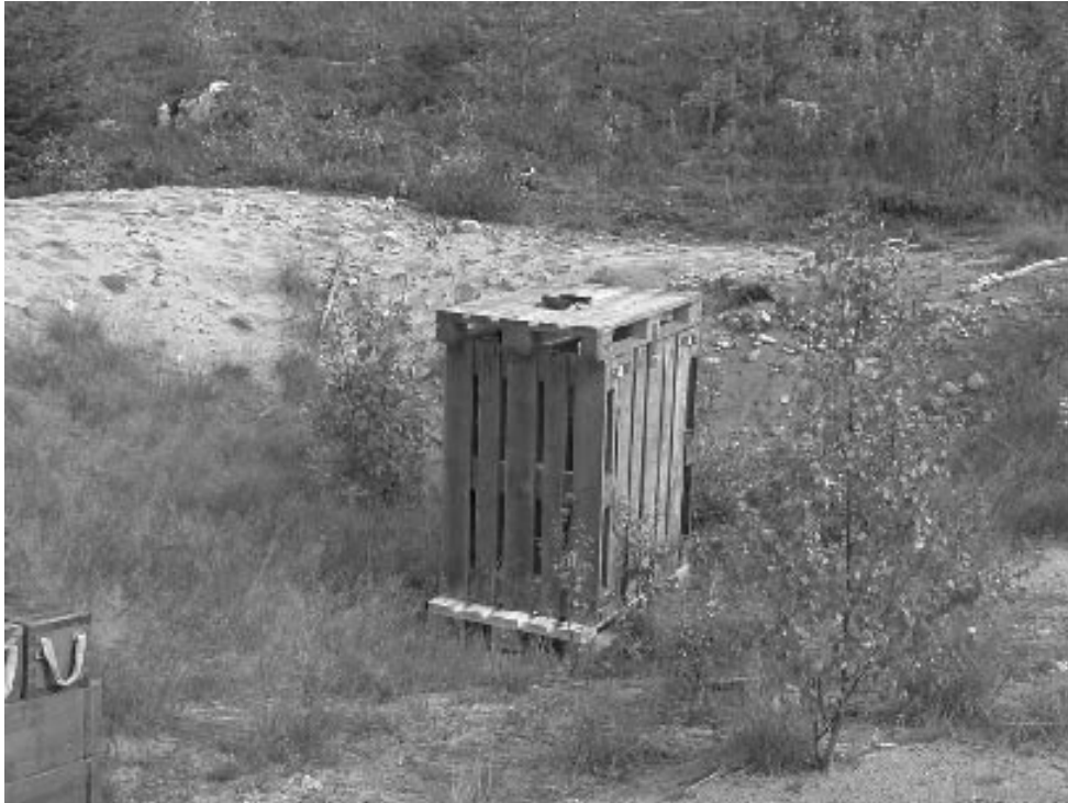
Fig 9. Sources were placed within physical barriers to prevent people and animals to come too close to the sources. Some of the sources were placed in wooden cages. The picture shows the wooden cage for source 1:1 containing 4.9 GBq Co-60. The shielding is not yet applied. The source is manoeuvred with a rod through one of the slits in the cage.
