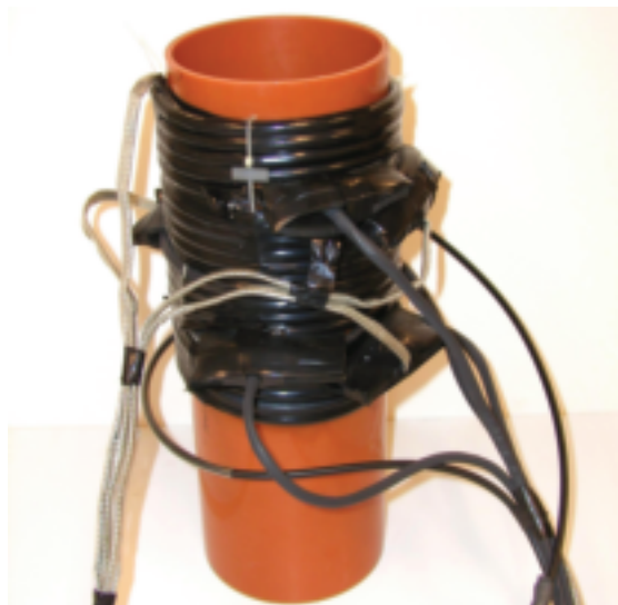
Figure 13: High voltage transmission line transformer based on cable technology.
