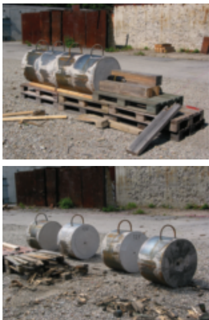
Figure 24: Photo from before a test with shaped charge against concrete, and after the test where each segment is inspected concerning damage and penetration.
