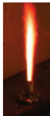
Figure 2: Burning of a smokeless ADN rocket formulation
