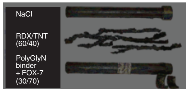
Figure 1: Detonability test on NaCl (inert reference), COMP-B and FOX-7/GAP
