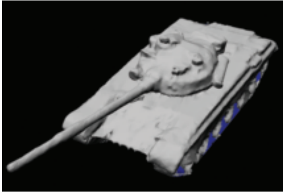
Figure 20: A computed 3D-model of the MBT, from the image data in figure 19. Some inconsistencies remain due to low resolution scanning (blue).
