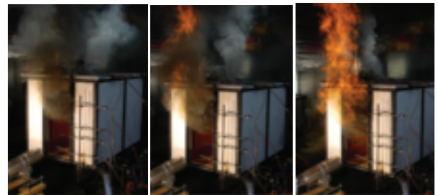
Figure 23: Flashover in model-scale fire test.
