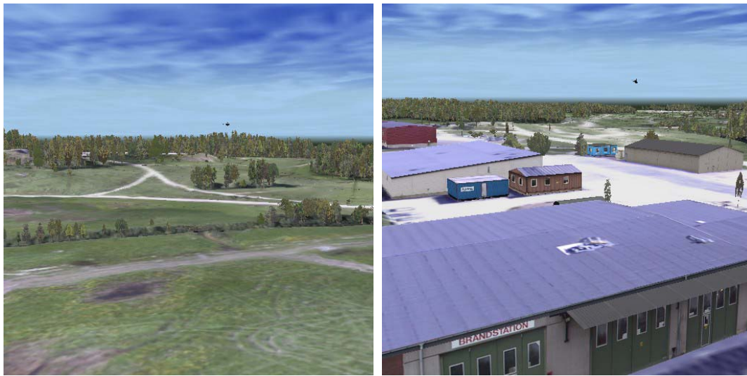
Figure 4: Synthetic scene in 3 D generated with the help of an airborne scanning laser radar (Top Eye) and data fusion with photography. Images FOI Dpt of Laser systems.
