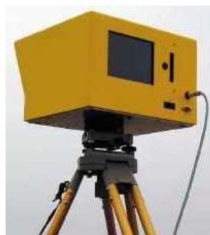
Figure 7: ILRIS 3 D laser scanner and key system parameters.
