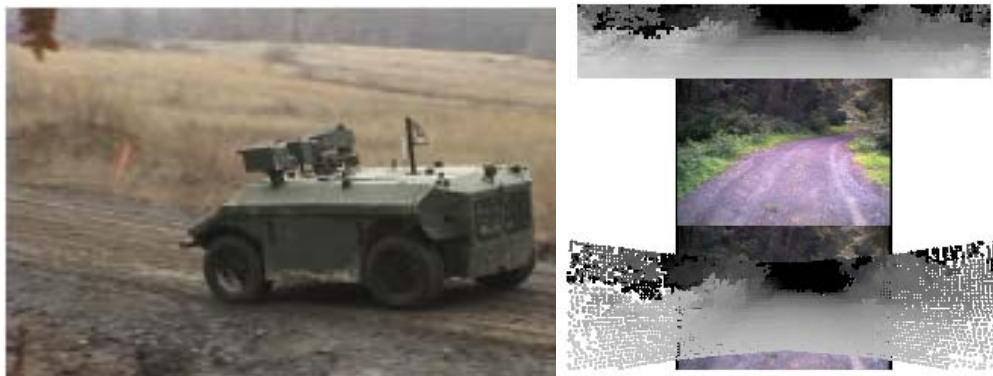
Figure 16: Left a test UGV for autonomous navigation. Fused laser range and CCD imagery. From Rasmussen 15 .
