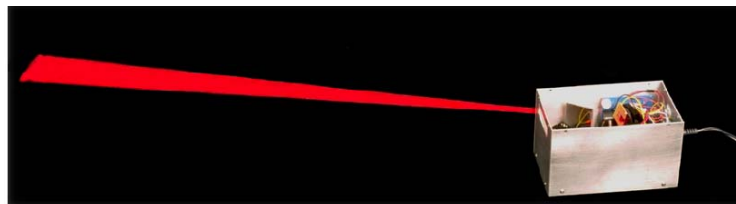
Figure 91: Lightweight, low power and low cost scanner based on optical MEMS technology dev. By Lockheed Martin.
