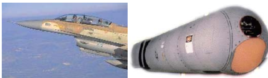
Figure 81: An Israel Air Force/Lockheed Martin F-16D equipped with a Rafael Litening I targeting pod. The pod contains a gen. III (3-5micron) FLIR, with a 640x480 digital detectors array. This system is also equipped with a target marker, which improves the coordination of ground and air forces, by designation of targets by day or night. Litening III system is also equipped with a dual-wavelength diode-pumped laser for ranging and designation.
