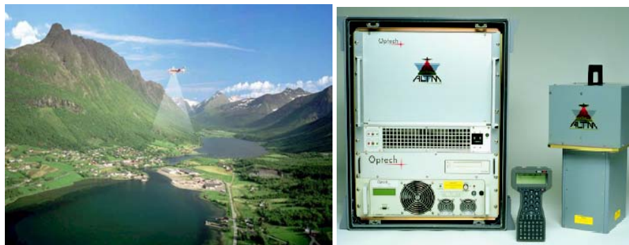
Figure 3: Example of a commercial lidar for airborne terrain mapping, ALTM from Optech, Canada.
