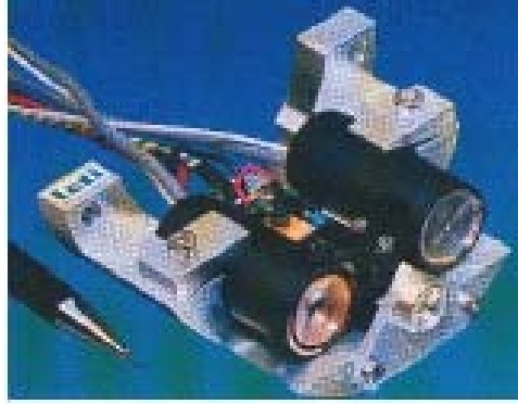
Figure 87: Compact laser radar for car applications developed by Leti in France.
