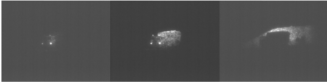
Figure 53: Gated viewing images of a terrain vehicle target at a distance of 7.2 km. Left: The front of the target is inside the gate. Centre: The entire target is inside the gate. Right: The gate is behind the target. The bottom part of the target is occluded by the foreground. Images FOI.
