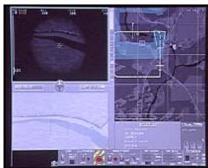
A typical ELVISS screen presentation, showing the same area viewed by the two sensing systems, geographic reference data and the operating controls and parameters for the system.
