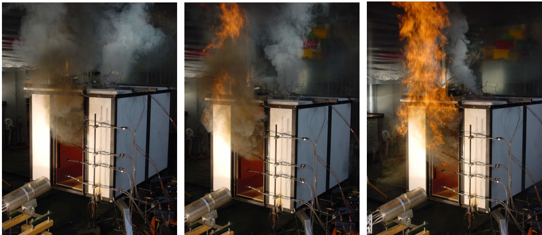
Figure 3-1 Flashover sequence from test C6.
