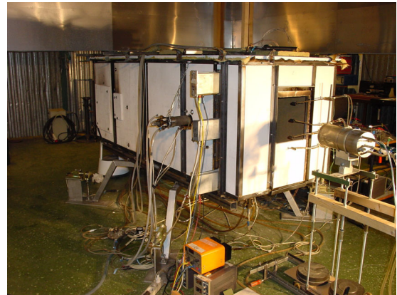
Figure 2-7 Illustration of the experimental geometry to study horizontal fire spread between compartments.
