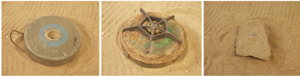
Figure 12. From left to right are the three investigated objects: the low metal content AT mine, the metal AT mine and the stone.
