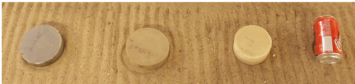
Figure 13. The objects tested to resemble AP mines and similar sized objects. The three first objects are made of steel, beeswax, and styrofoam, respectively, and the last object was an empty soft drink can.
