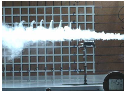
Figure 10 – Smoke injected to hit turbine disk at 10 o'clock
