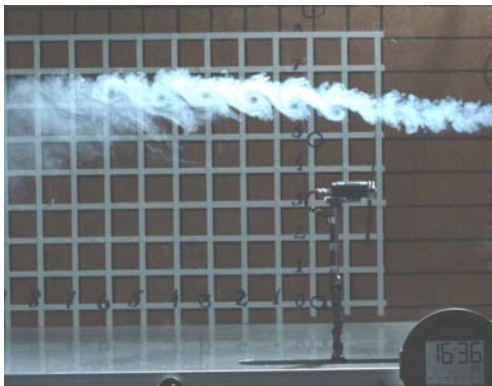
Figure 9 – Smoke injected to hit top of turbine disk
