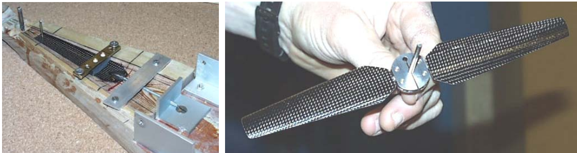
Figure 3 - The blade placed in the mould for attachment of the pitch axis (left). A complete rotor with two blades mounted to the hub (right).
