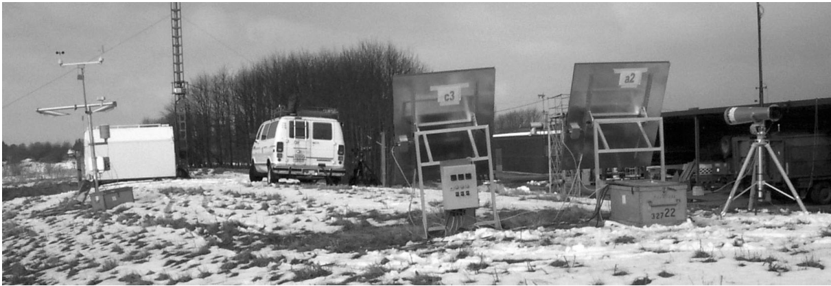
Figure 6 An overview of the measurement set-up. From left: weather station, sensors, panels and ambient air temperature reference.
