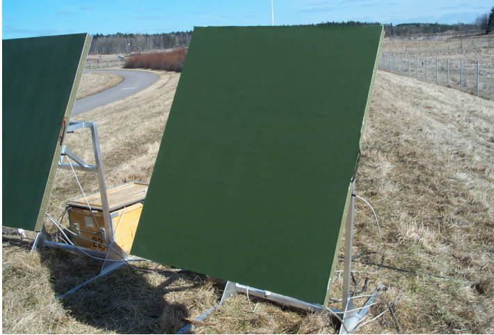
Figure 2 The two dark green panels on stands: painted (left) and low emissive foil (right).
