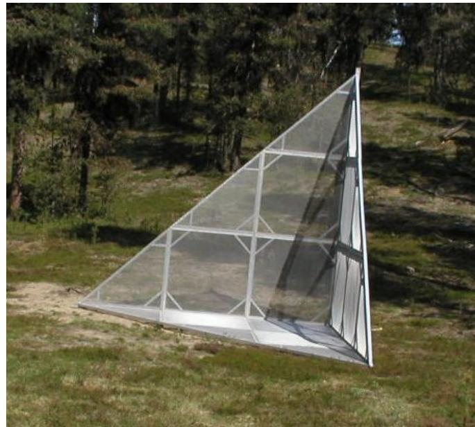
**Figure 26. Trihedral radar reflector with short side of 5 m. (ID = 1)**
