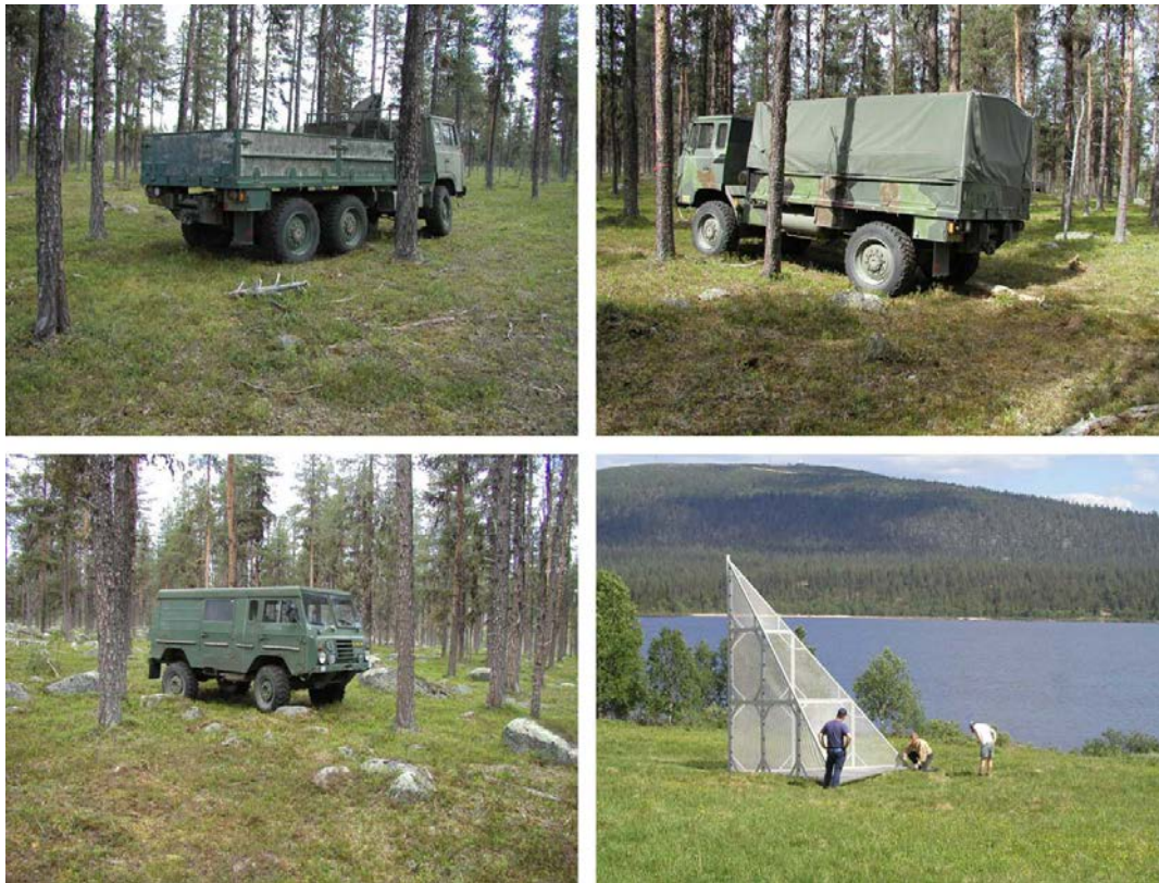
Figure 7. The terrain vehicle models TGB40 (upper left), TGB30 (upper right) and TGB11 (lower left). The deployed trihedral in Nausta (lower right) was adjusted for each flight pass to allow radiometric calibration.
