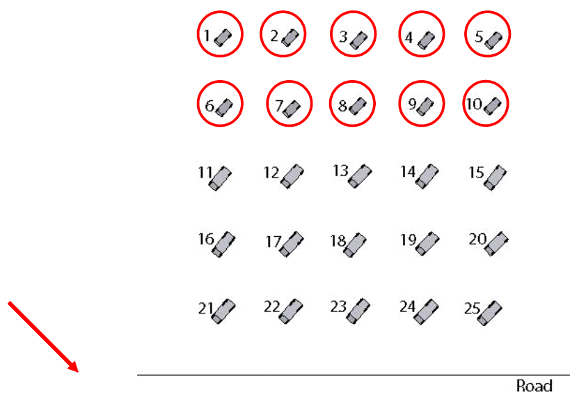
Figure 22. Imaging geometry for one pass used in study number 1. The arrow indicates the flight heading. The geometry resulted in all 10 small targets (enclosed by circles) to have an end-on orientation.
