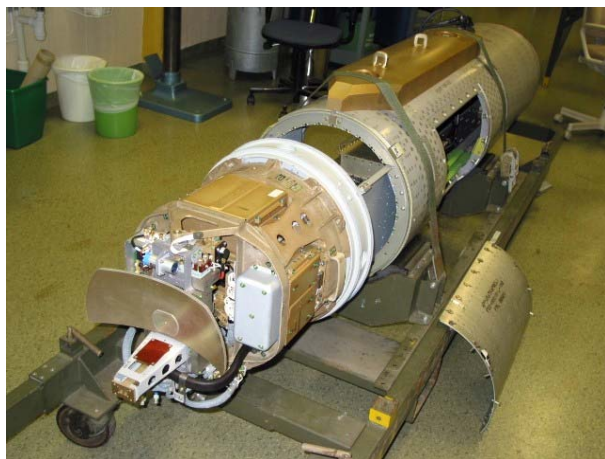
Figur 3. GMS. Apparat 64 monterad i pod
