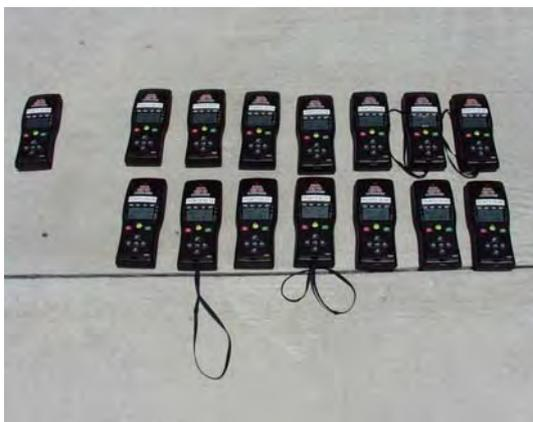
Figure 4: GPS receivers during initialization and calibration. (Photographer Markus Axelsson)
