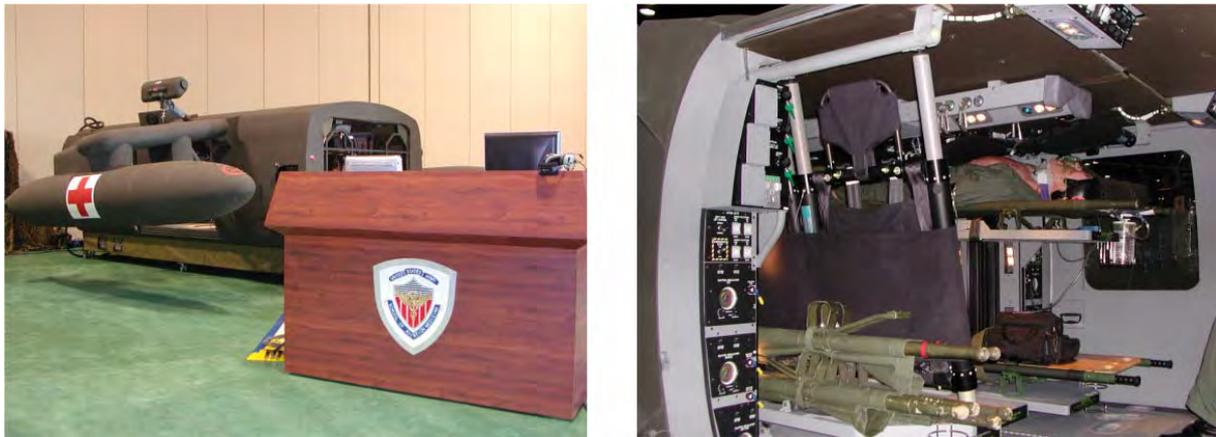
**Figure 3:** MST trainer exterior view with the instruction and observation console (left) and the interior view of MST displaying litters and on-board equipment (right). (Photographer: Mona Crissey)
